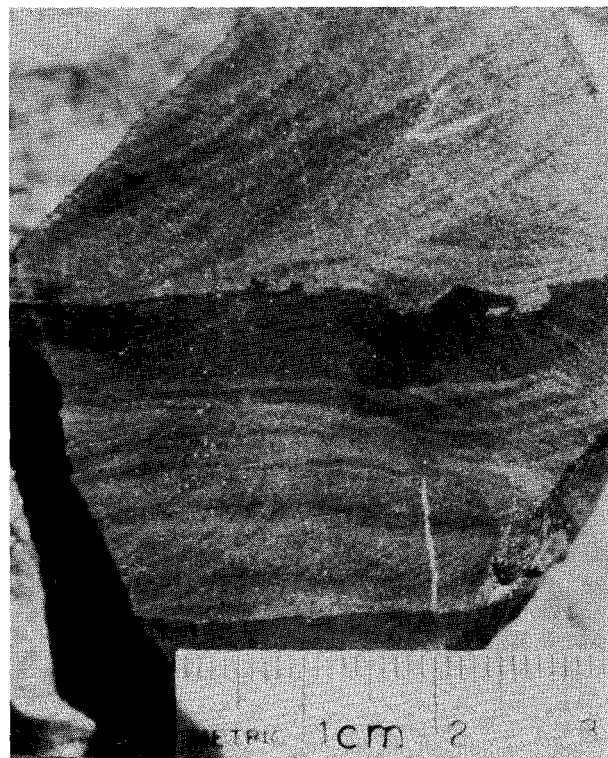
Figure 17. Graded cycle in banded argillite (pJa). Note preserved load casts.
