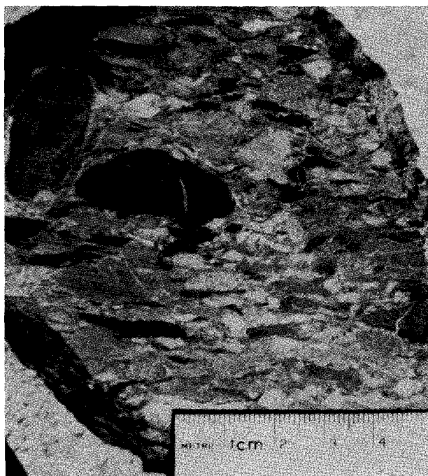
Figure 18. Intraformational conglomerate consisting chiefly of rounded and stretched mud clasts (pJa).
