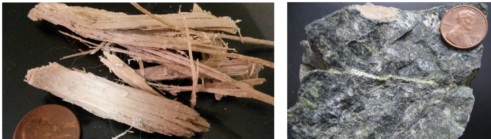
Tremolite collected from a marble unit near Fairbanks, Alaska (photograph taken 10/01/2014 by J.E. Athey). Serpentinite with thin asbestos vein. Sample collected from between the villages of Manley Hot Springs and Tunana in the Tunana A-3 Quadrangle, Alaska, by P.A.C. Burns. Photo taken by D.N. Solie. Approximate location 65.121322°, -151.024601° (WGS84).
