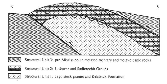
Figure 2. Schematic cross section through the Jago stock region showing structural stratigraphy and essential structural relationships.
