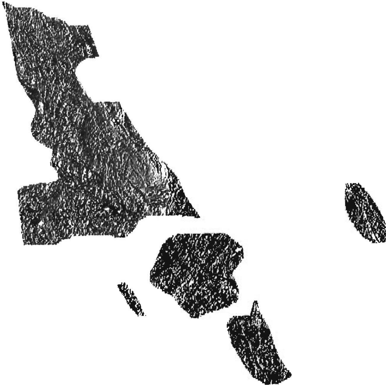
Figure 3: Shadow map of the aeromagnetic data from the Stikine area, Southeast Alaska. Illumination source is at 282 degrees. High magnetic values appear like the tops of mountains that are hit by sunlight.
