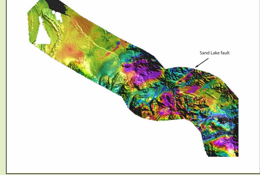
Figure 9: The aeromagnetic values for the western portion of the survey area are shown draped over the digital terrain model (DTM) computed by Fugro Airborne Surveys from the data. High values are represented by purple and magenta; low values by black and dark
