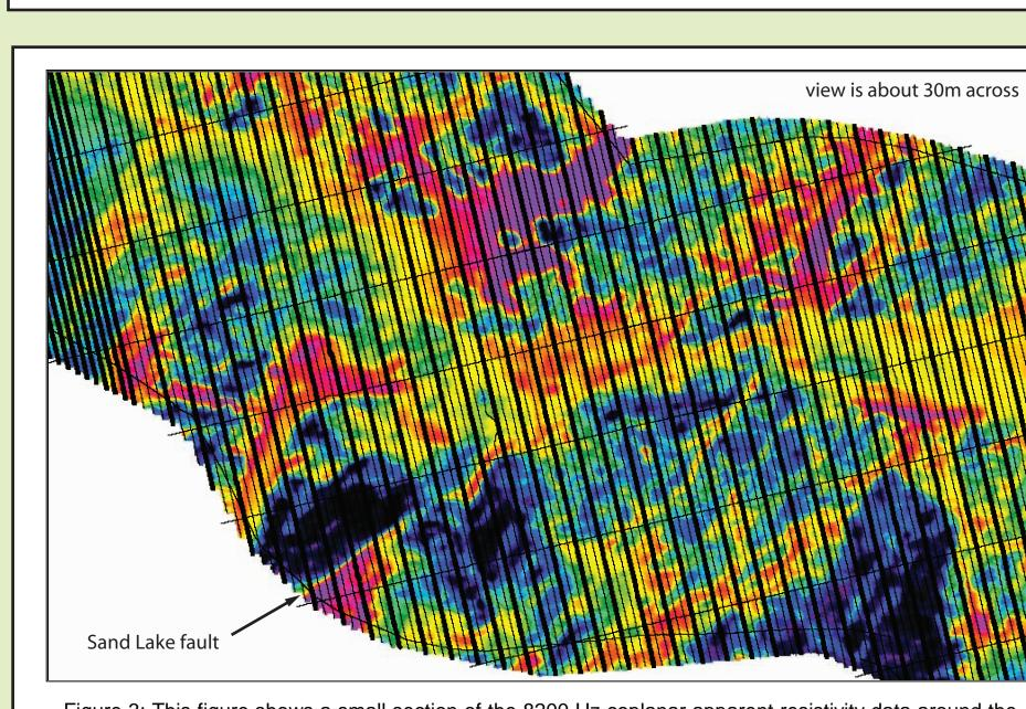
Figure 3: This figure shows a small section of the 8200 Hz coplanar apparent resistivity data around the Sand Lake fault area with traverse, tie, and boundary lines shown in black. Traverse line direction and spacing were N10°W and ¼ mile (0.4 km) respectively; tie lines were perpendicular to flight lines and were spaced about every 3 miles (5 km). Black and blue represent highly resistive units and magenta and purple represent highly conductive units.
