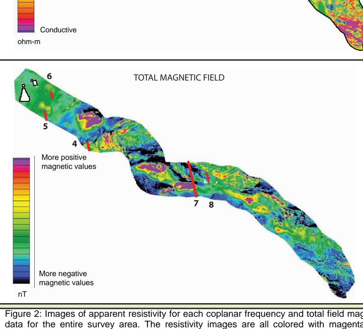
Figure 2: Images of apparent resistivity for each coplanar frequency and total field magnetic data for the entire survey area. The resistivity images are all colored with magenta and purple as most conductive and black and blue as most resistive. Maximum and minimum values (ohm-m) for each frequency differ, as well as color distributions. Most color schemes shown approximate the equal area color scheme, where an equal number of values are shown for each color.
