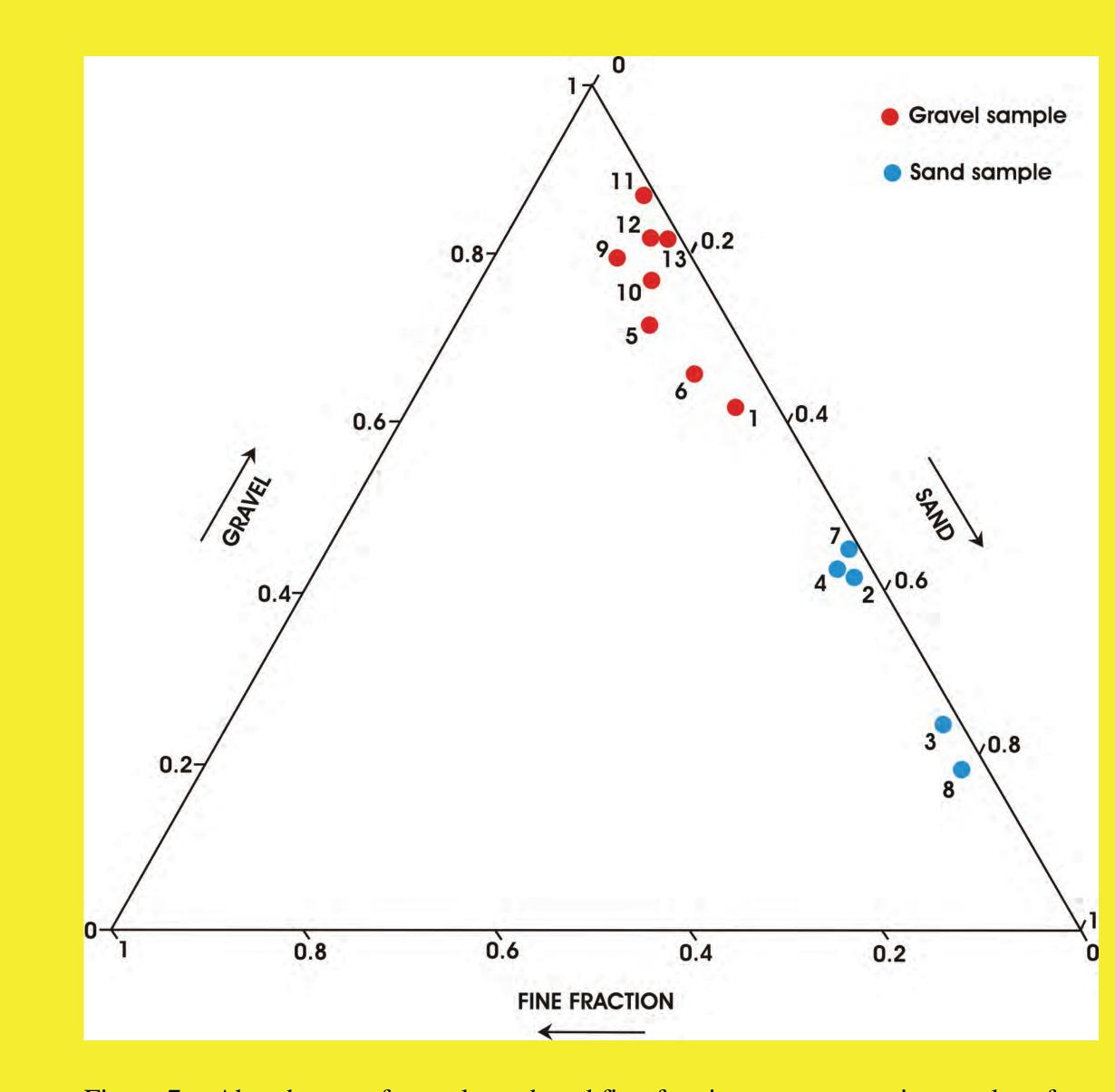
Figure 7. Abundances of gravel, sand, and fine-fraction components in samples of gravel and sand beds in south and west walls of M.S. 62-2-005-2 (table 1), northeastern Tok fan, Tanacross B-4 Quadrangle (locality A).
