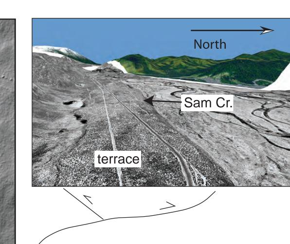
3D flyover view using lidar intensity image in ArcGlobe. Inferred structural model shown below image. South-dipping thrust fault and north-dipping back thrust have warped an outburst flood terrace.
