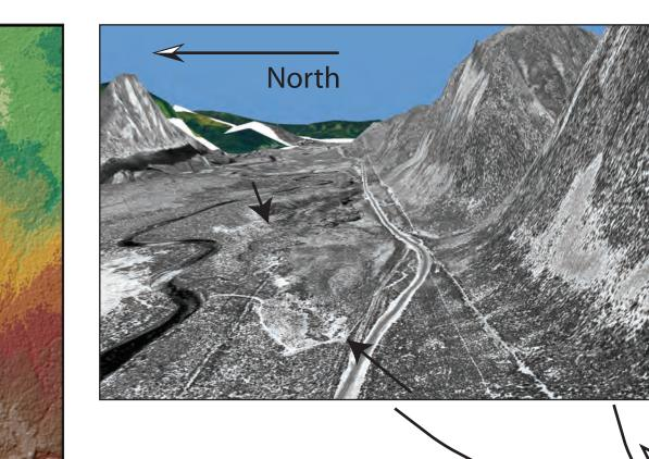
3D flyover view using lidar intensity image in ArcGlobe. Inferred structural model shown below image. Imbricate thrust faulting has created triangular facets along the range front and a Holocene fault scarp north of the range.
