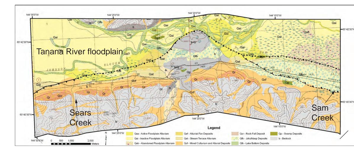
Geologic map along the Dot "T" Johnson fault modified from Reger et al., 2008-3a. Geologic mapping indicates that the trace of the fault has been eroded along the margin of the Tanana River floodplain. The fault cuts alluvial deposits and outburst flood deposits in the vicinity of Sears Creek and Sams Creek, respectively.
