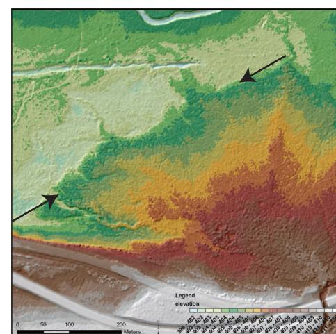
A hillshade map illustrates the cont between the uplifted and warped alluvial fan and the undeformed floodplain to the north.
