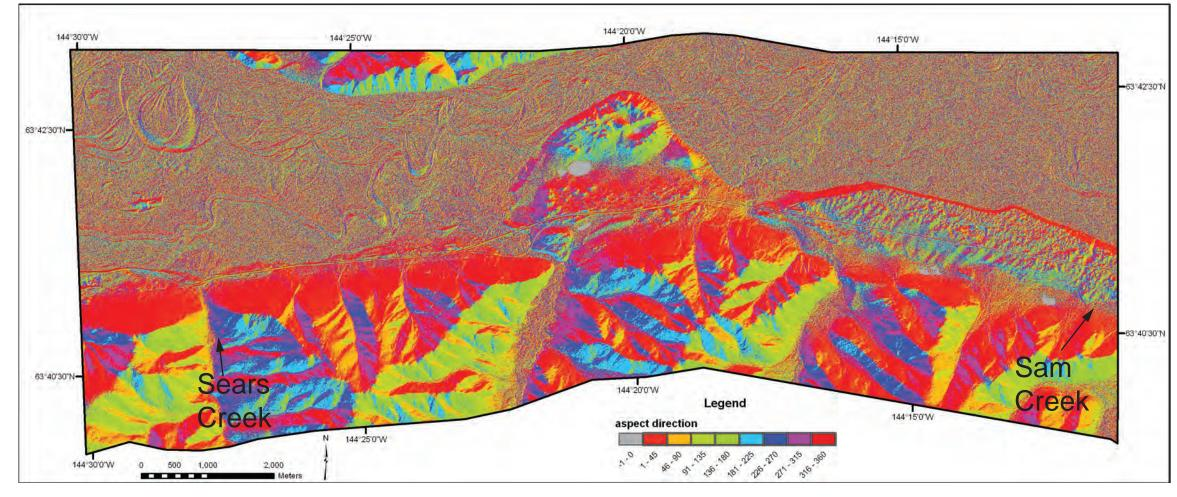
Aspect maps can be created to illuminate specific slope aspects. Here the color ramp supports our interpretation that the outburst flood deposit terrace at Sam Creek is warped on the hanging wall above a north dipping back thrust fault (See section 5, 3D view of Sam Creek).
