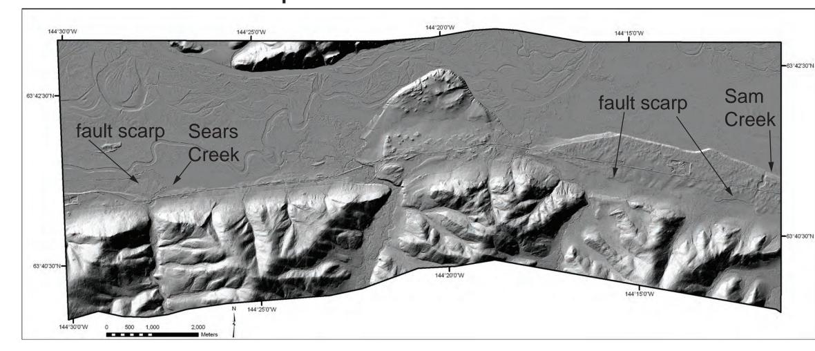
Bald earth hillshade models have become the industry standard base maps for pipeline design and construction, as well as neotectonic research. By interpreting hillshade models, steep terrain, landslides, floodplain configuration, areas of permafrost, and tectonic geomorphology can all be rapidly mapped and evaluated. In this map, fault scarps at Sears Creek and Sam Creek are easily recognizable.
