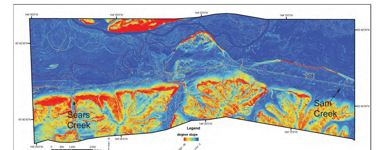
Slope maps are useful for detecting fault scarps in areas of low relief. Scarps may be expressed as lineations of bright color due to their significantly steeper faces as compared to the surrounding topography.
