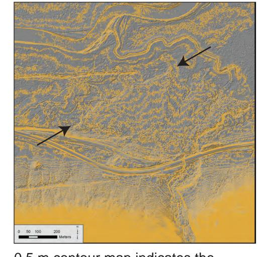
0.5 m contour map indicates the presence of fault scarp shown between arrows.
