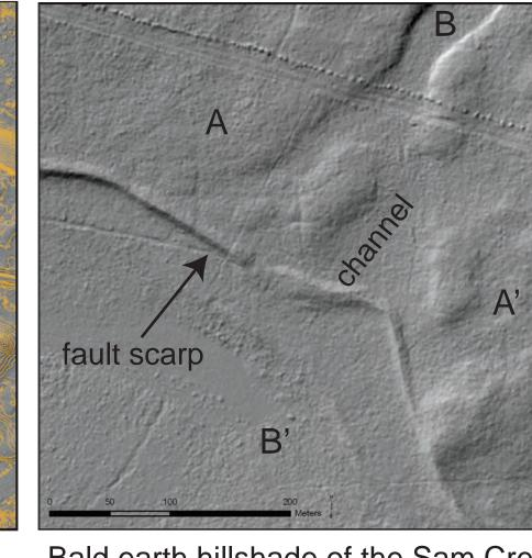
Bald earth hillshade of the Sam Creek site showing the abandoned channel of Sam Creek isolated by uplift on a north dipping backthrust.
