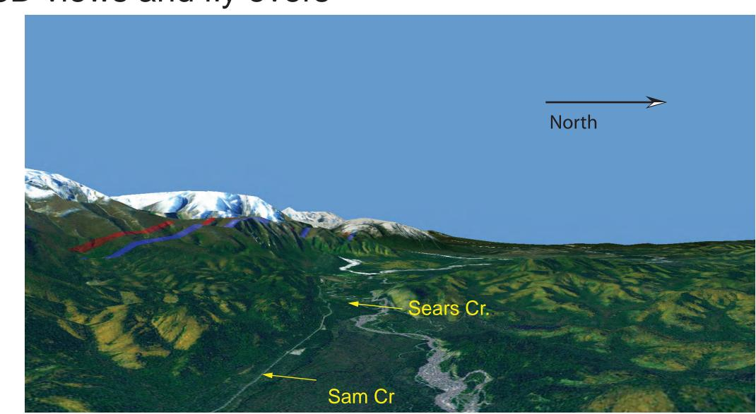
View west along the Dot "T" Johnson fault between Sam and Sears Creeks. Image produced in ArcGlobe using 60 m digital elevation model. 3D views and fly overs can be extremely useful in conveying geologic hazard observations to pipeline project engineers and managers. Images can be viewed from multiple angles to highlight specific features.
