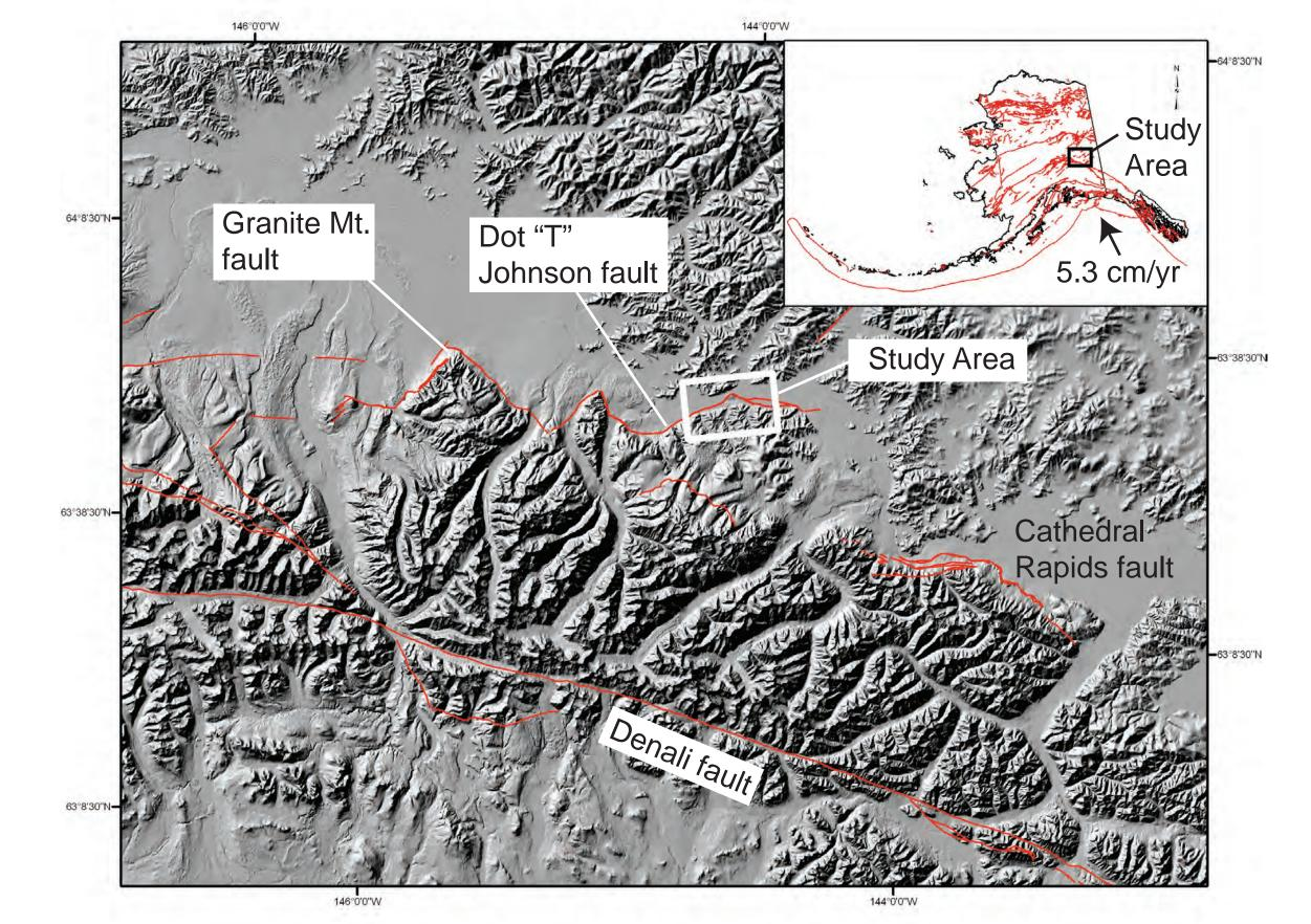
Hillshade of the Alaska Range showing the Denali fault and thrust faults that bound the north side of the range. Inset shows location of study area relative to Alaska and the distribution of faults. Only a fraction of these faults have been documented to have Quaternary deformation (See poster # 30-1 this session).
