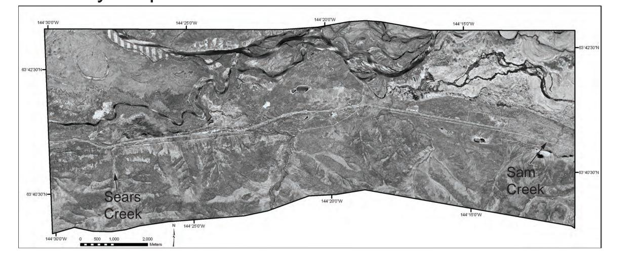
In areas with poor air photo coverage, intensity maps can be derived from lidar point cloud data. Intensity maps can highlight subtle differences in Quaternary geologic units and their surface reflectance intensities. The ease of creating intensity images in ArcMap allows the user to generate air photo "like" images rapidly over broad regions.
