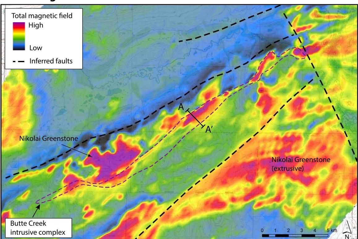
New aeromagnetic data (GPR2014-1; Burns et al, 2014) highlights only the most mafic (and serpentinized) portions of the Butte Creek intrusive complex; magnetic highs reflect the distribution of the upper, high-TiO, member of the extrusive Nikolai Green-
