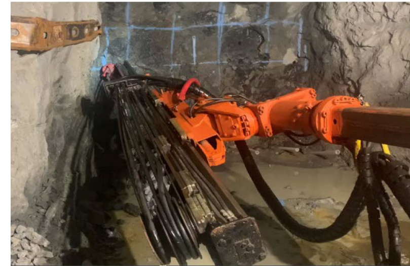
Advancing towards Lucky Shot vein with footwall drift parallel to the vein
