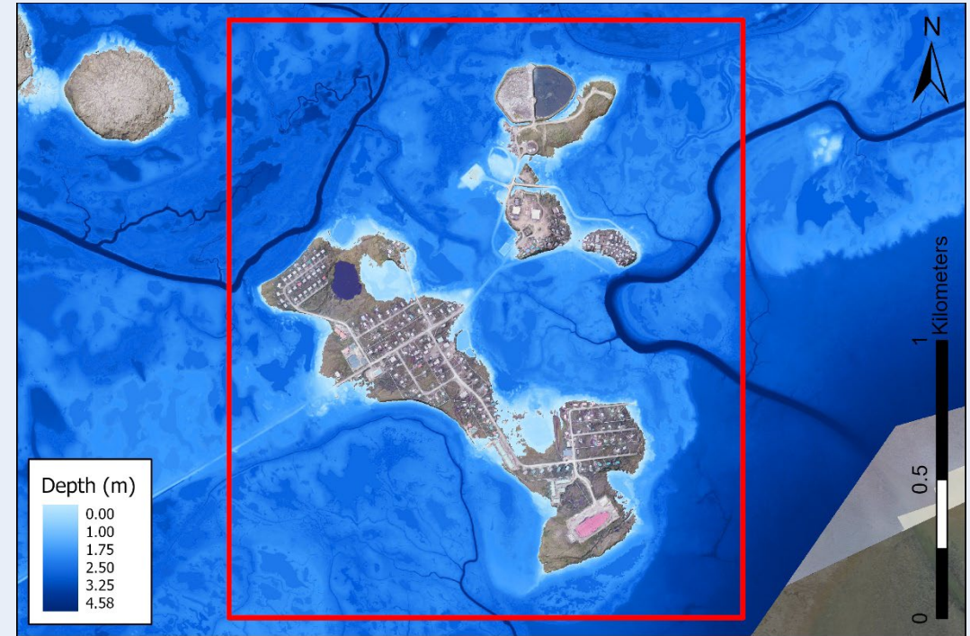
Modeled flood inundation from Extratropical Typhoon Merbok, 2022, in Hooper Bay, AK
