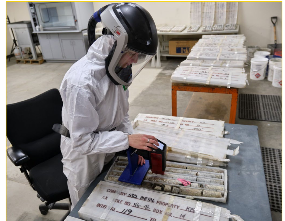
GMC staff curating and XRF scanning Bokan core.
