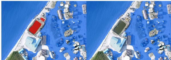
Figure 1. Comparison of a simple bathtub inundation model (left) and a hydrologically connected bathtub model (right) in Teller, Alaska. The area in blue is hydrologically connected to the inundation source, whereas the areas in red are protected by barriers and incorrectly depicted as inundated in the simple bathtub model.
