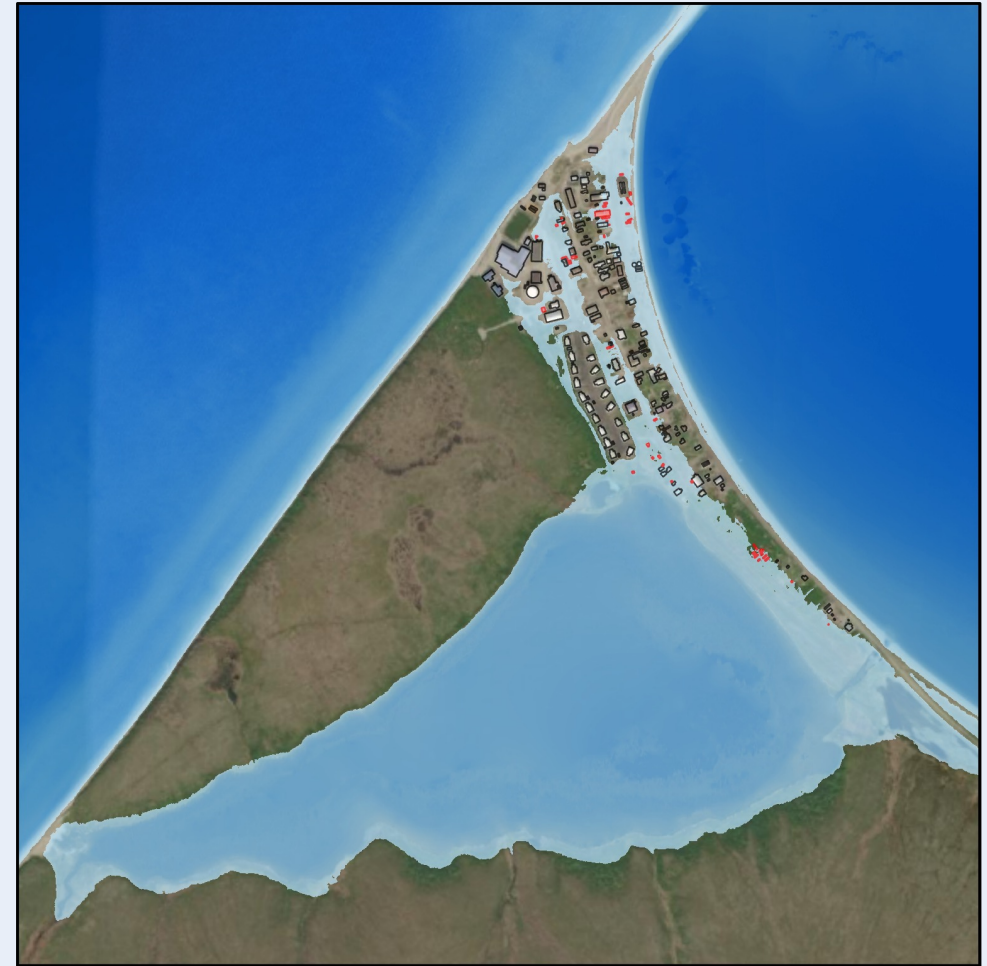
Still water inundation model (SWIM) for Teller, AK, at 2.75 m (NAVD88)
