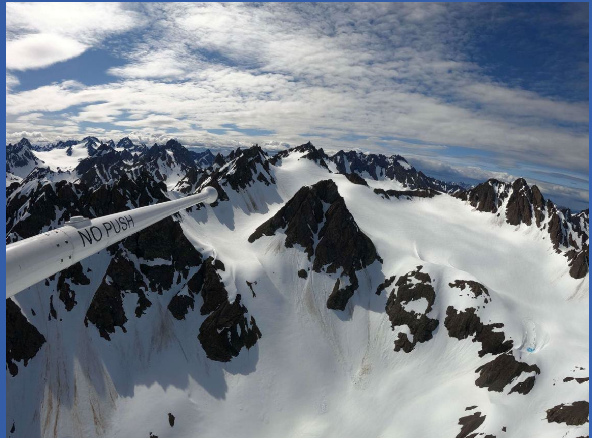
Magnetometer beneath helicopter on survey in the Kilbuck Mountains.
