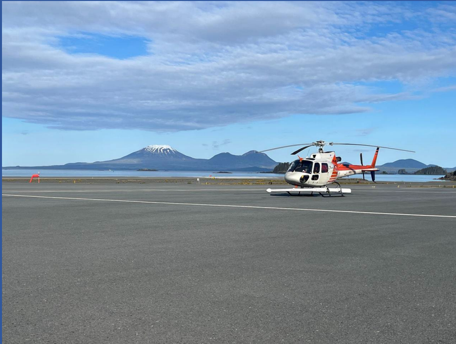
Helicopter with airborne magnetometer (large Q-tip)
