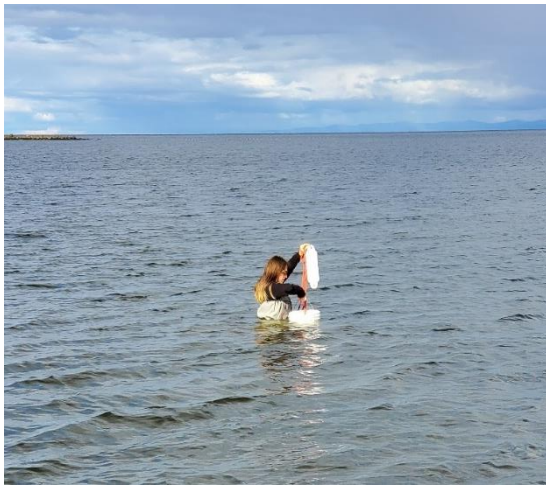
Figure 2. Solinst Levellogger installation offshore near Saint Michael, Alaska.
