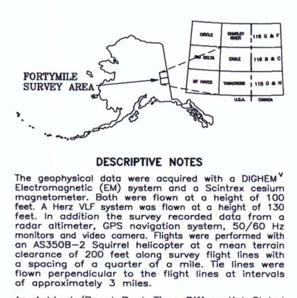
An Ashtech/Racal Real—Time Differential Global Positioning System (RT—DGPS) was used for both navigation and flight path recovery. The helicopter position was derived every 0.5 seconds using real—time differential positionina to a relative accuracy of
