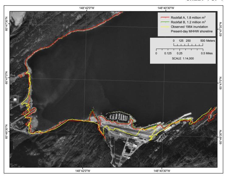
Modeled potential inundation by the rockfall-generated waves, for two different cases. The volume in Rockfall A is 1.8 million m3 (63 million ft3) and in Rockfall B is 1.2 million m3 (42 million ft3). The DEM corresponds to the present-day MHHW datum. Because of the steep topography, inundation areas for several tsunami scenarios have a common boundary, and the plotted extents of the inundation areas may overlay each other.
