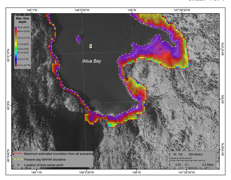
Maximum composite potential inundation resulting from all scenarios in the southern part of Iktua Bay, and the maximum composite flow depths over dry land. Large uncertainties in the DEM in Iktua Bay could severely degrade the accuracy of numerical results. The present-day MHHW shoreline is shown by a dashed yellow line.
