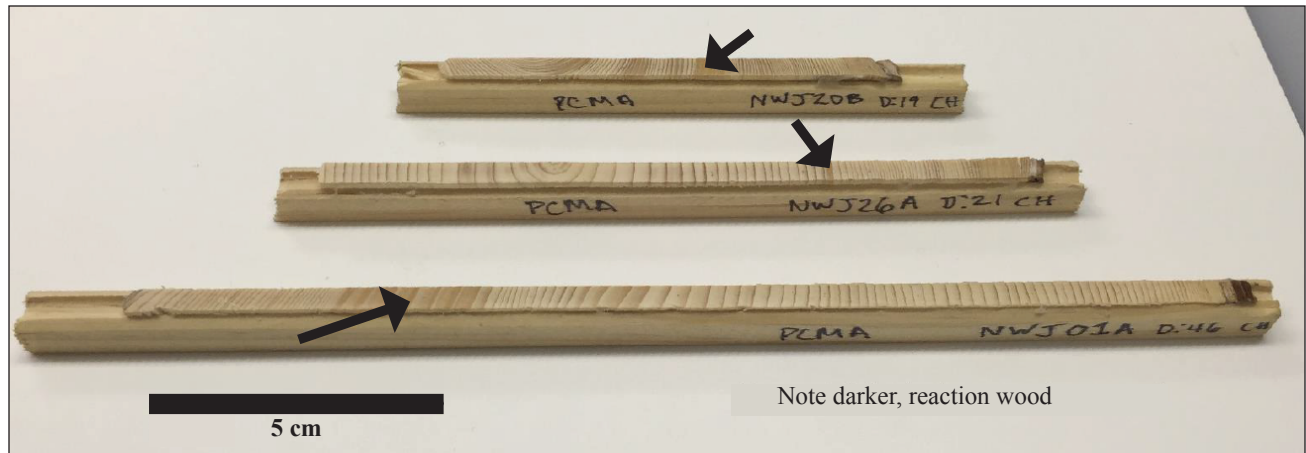
Figure 7. Three samples highlighting reaction wood in three separate trees. Arrows point out sections of reaction wood (darker than surrounding sections).
