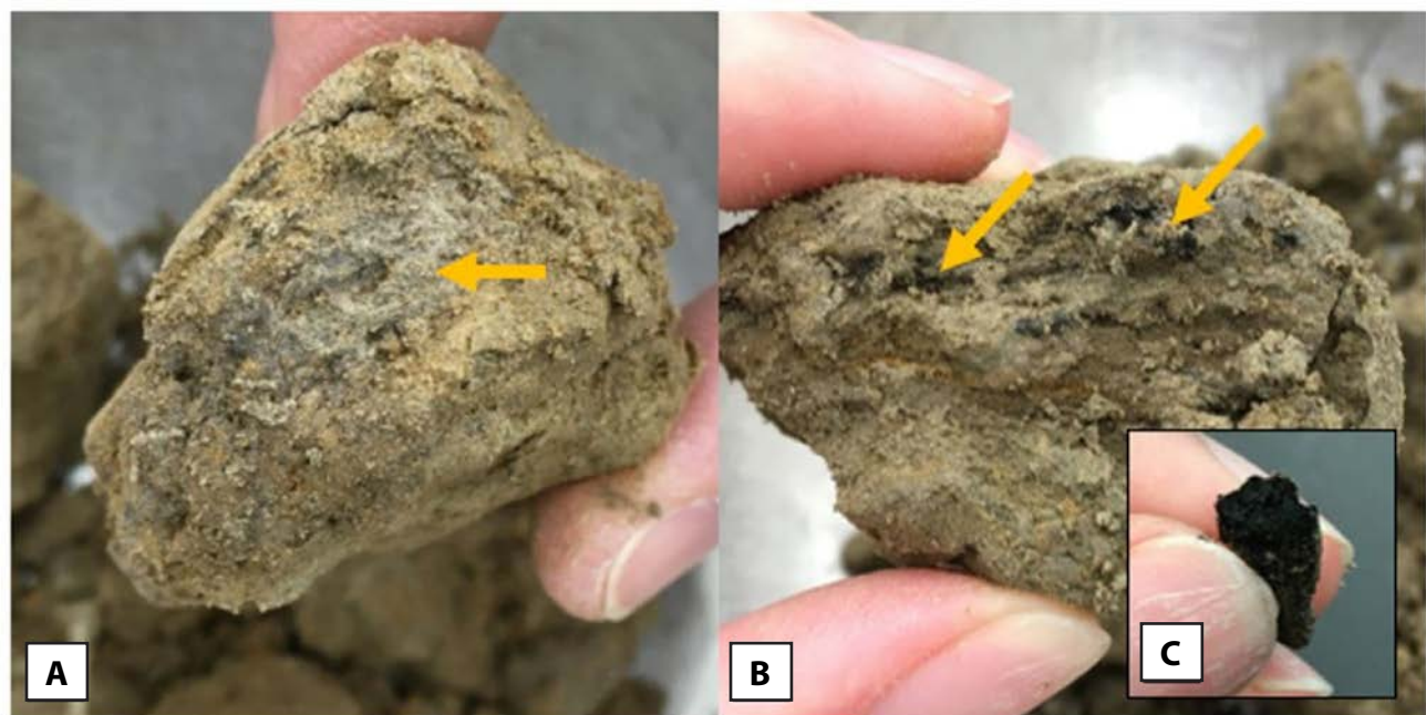
Figure 7. Photos of organic samples submitted for radiocarbon dating. A. TH06 paleosol layer (indicated by arrow). B. TH08 charcoal pieces within the soil mass (indicated by arrows). C. TH08 charcoal piece extracted from the soil.
