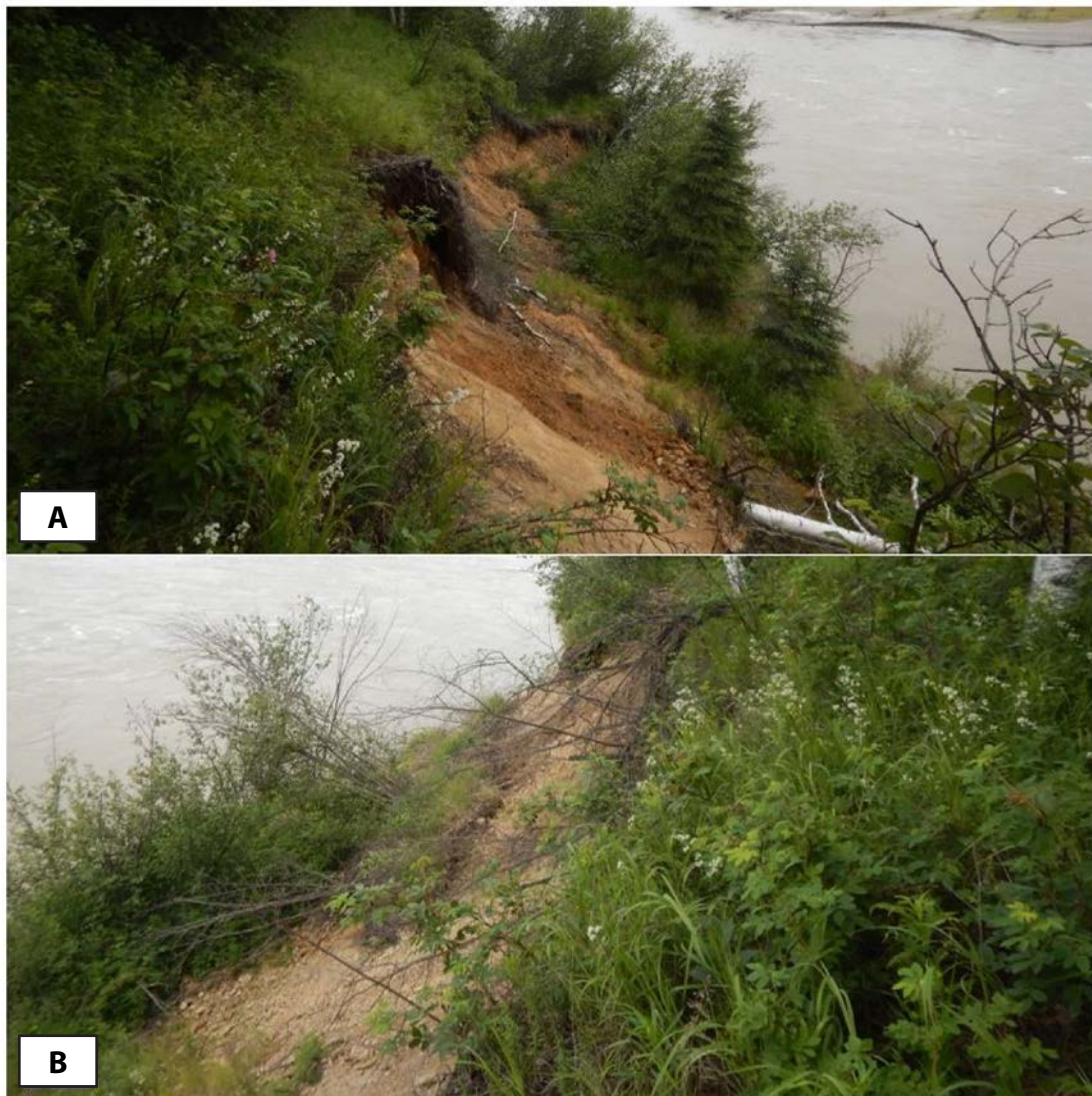
Figure A46. Images of BigB5_7S_7E_20_SW7 from July 2, 2020. A. View of the fresh soil exposed at the head scarp to the east, and (B) view of the head scarp with exposed soil to the west. Photographs taken by MD.
