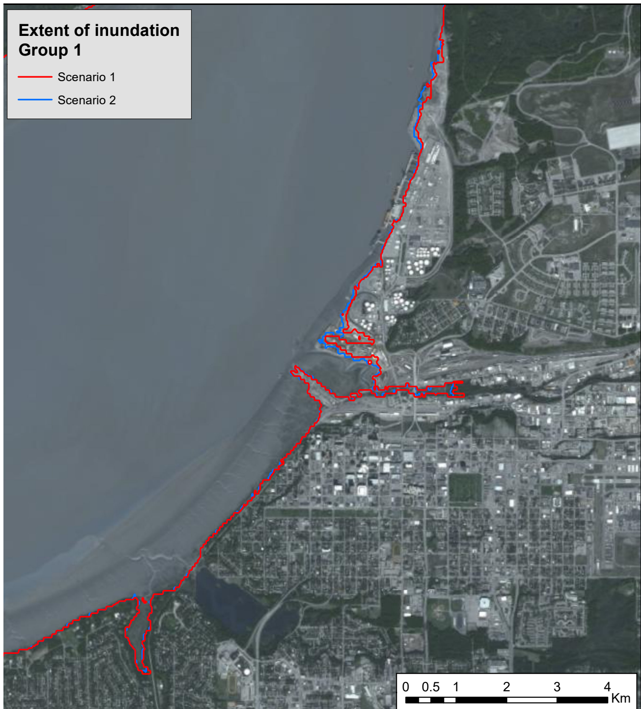
Figure 15A. Tsunami inundation in downtown Anchorage for group 1 scenarios.
