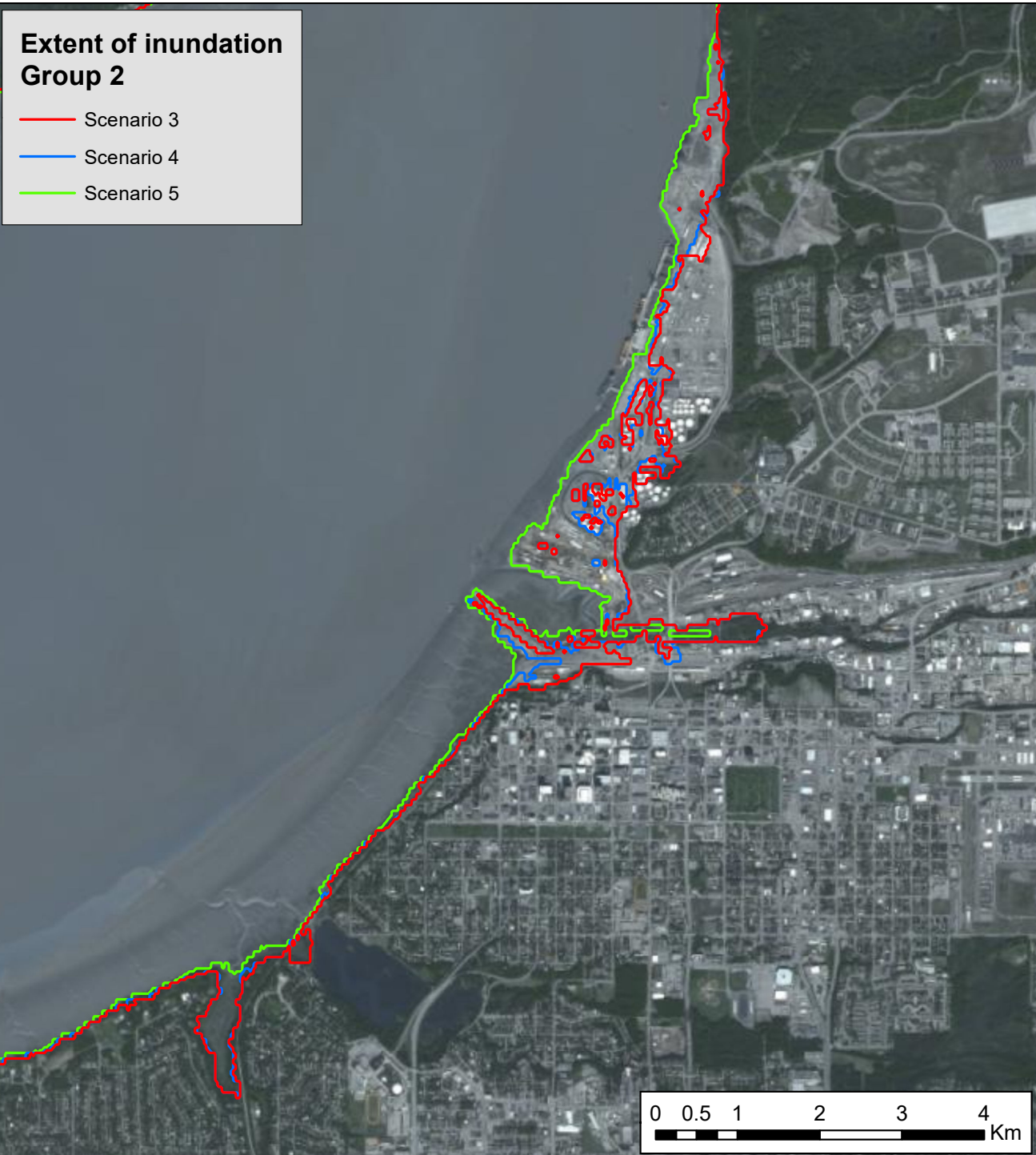
Figure 15B. Tsunami inundation in downtown Anchorage for group 2 scenarios.
