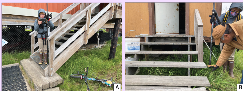
Figure 10. GNSS observations of reported heights of the flood event on December 14, 2015, in Kipnuk, Alaska. Water levels reached 3.9 ft (1.18 m) MHHW at the bottom stair of the council building (A) and 4.1 ft (1.25 m) MHHW at the second stair of Tim Swanson's home (B).
