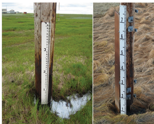
Figure 1. Flood staffs installed in Kwigillingok, Alaska, in 2017 (left) and 2023 (right).
