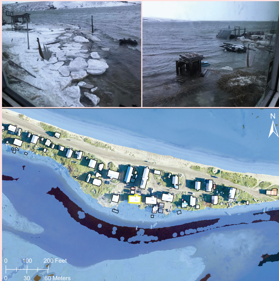
Figure 15. Photographic evidence (top) of flooding south of residence (yellow) in the 2016 orthoimagery, overlaid with a simple bathtub model applied to the 2015 DTM simulating a water height of 4.7 ft (1.44 m) MHHW to approximate the flooding depicted.
