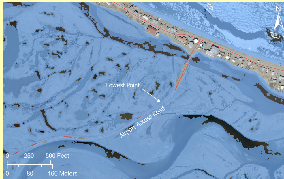
Figure 9. Airport access road within the 2013 orthoimagery overlaid with a simple bathtub model applied to the 2015 DTM simulating a water height of 3.9 ft (1.19 m) MHHW.
