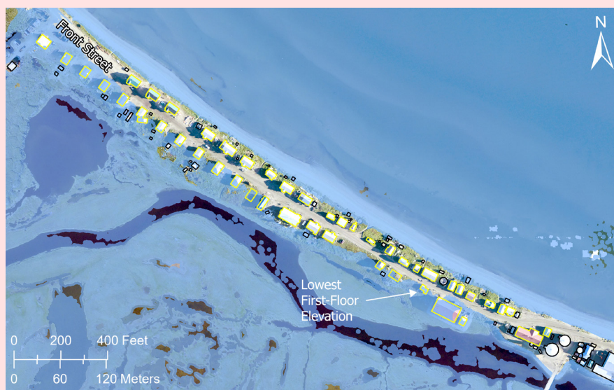
Figure 17. Occupied buildings (yellow) in the 2016 orthoimagery, overlaid with a simple bathtub model applied to the 2015 DTM simulating a water height of 7.2 ft (2.18 m) MHHW to approximate the flooding described.
