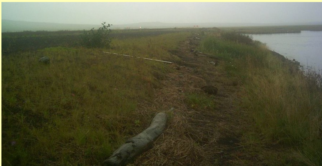
Figure 2. High water mark “strandline” along the southern edge of the airstrip in Stebbins, Alaska, associated with the October 2004 flood event and collected in August 2005 by Baker and Coastal (2007).
