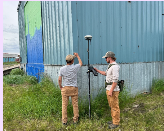
Figure 4. High water mark associated with the November 2013 flood event identified at the northeast corner of the old store in Stebbins, Alaska.
