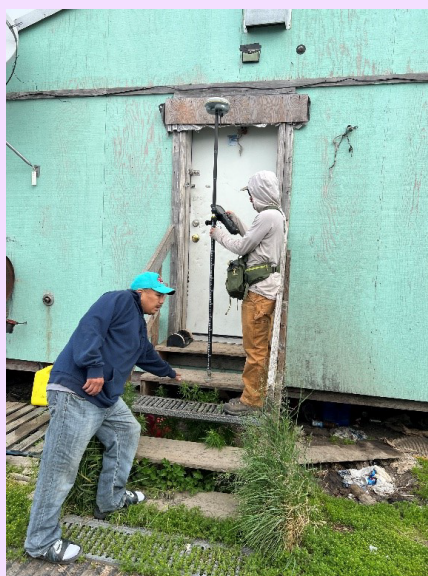
Figure 5. High water mark associated with the August 2019 flood event identified by a community member at the steps of a residence in Stebbins, Alaska.
