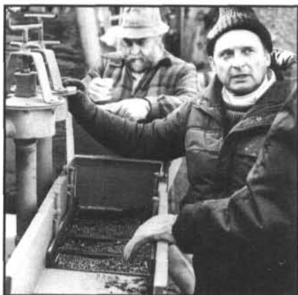
Figure 34. Efficient recovery is critical to the profitability of all placer operations. The owner and operator explains the action of the shot-loaded recovery boxes in his jig system. As the gravel is washed, heavy particles like gold sink through the ball bearings while lighter material is pulsed off. The gold is collected in the sump. (Photo by Bruce Campbell)
