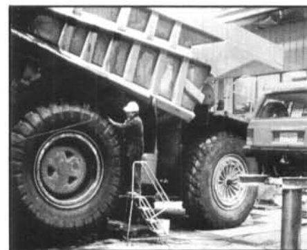
Figure 39. Part of the challenge of all-weather operations is equipment maintenance. In the Usibelli shop, mechanics service a 95-ton Dresser Haulpak truck. This truck can carry more coal than a railroad car. (Photo by Usibelli Coal Mine)
