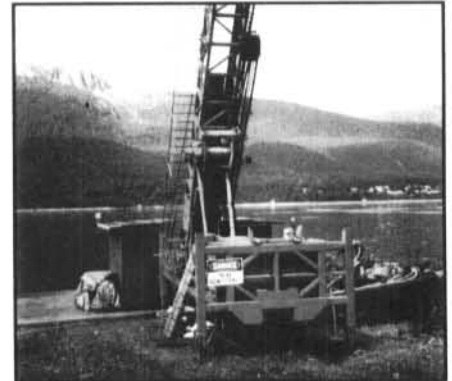
Figure 40. New technology is opening opportunities for Alaska. This 5,000-ft drill hole under Gastineau Channel near Juneau intercepted the Treadwell Mine structure far below the deepest workings. It is the deepest hardrock drill hole in the state and utilized the most sophisticated navigational drilling technology. At its prime, the Treadwell had many shafts drilled under the ocean. It ceased operations in 1922 when it was thought uneconomic to pump out its flooded tunnels. (Photo by R.C. Swainbank)
