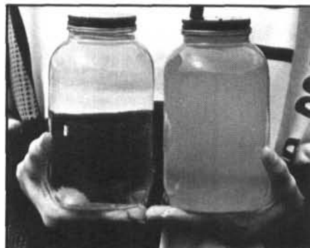
Figure 23. On August 26, 1989, samples were taken from the naturally turbid waters of Hoseanna Creek (right jar) and the clear discharge from the Usibelli settling pond (left jar). Usibelli Coal Mine made a major investment to bring discharged water to this required standard. (Photo by Usibelli)
