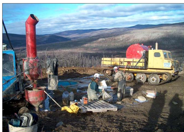
Figure 12. Reverse-circulation drilling by G.F. Back Inc. as part of Fairbanks Gold Mining Co.'s exploration of the Fairbanks mining district. Photo provided by Fairbanks Gold Mining Co.
