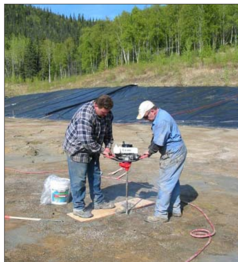
Figure 10. Auger drilling historic tailings at the Nixon Fork Mine for metallurgical and geochemical testing. St. Andrew Goldfields Ltd. plans to reprocess the tailings from past mining operations and recover additional gold. Photo provided by St. Andrew Goldfields Ltd.
