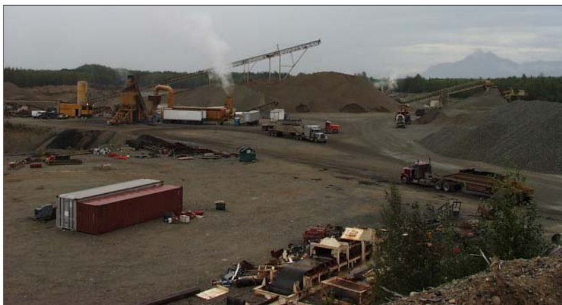
Figure 31. Quality Asphalt's sand and gravel operation north of Wasilla. Sized product is loaded directly into railroad cars for transport to Anchorage. Photo by Rich Hughes.
