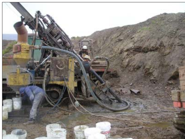
Figure 34. Reverse-circulation drilling at Rock Creek deposit near Nome. Photo provided by NovaGold Resources Inc.
