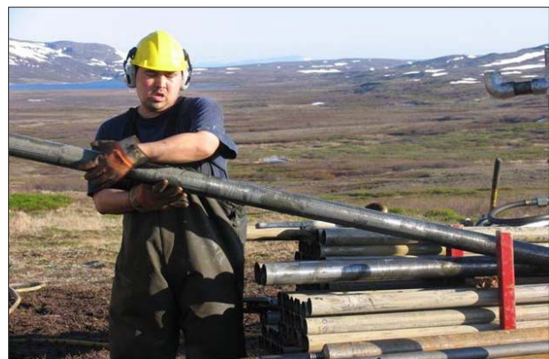
Figure 16. A driller wrestles with drill pipe at the Pebble property. Drilling is the dominant exploration tool used to identify mineralization in this region of Alaska. Photo courtesy of Northern Dynasty Minerals Ltd.
