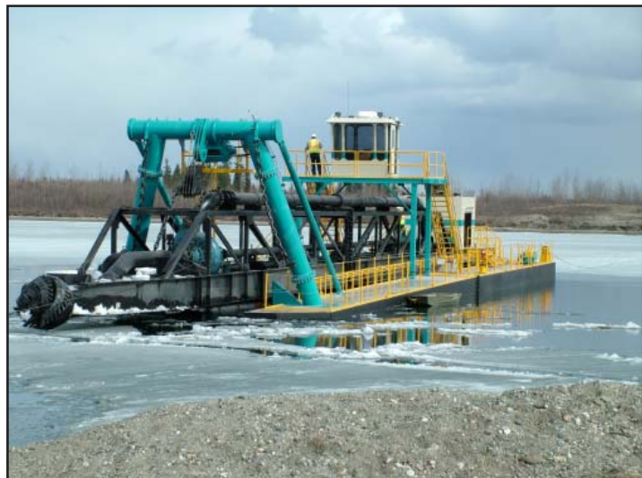
Figure 24. Floating dredge acquired by Exclusive Landscaping & Paving Inc. to extract sand and gravel. The 204 Marlin Dredge has a 16-inch intake pipe and can produce 500 to 1,000 tons of material per hour and can dig to a 100-foot depth. A two-man crew operates the dredge and it was commissioned at Exclusive's pit in the Fairbanks area during 2004. Photo provided by Exclusive Landscaping & Paving Inc.
