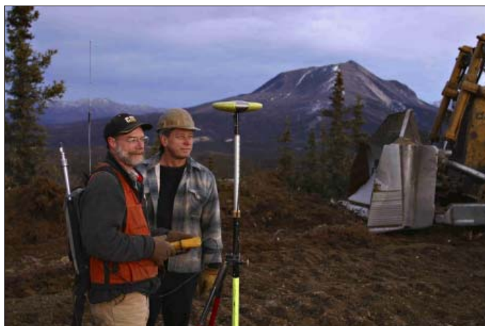
Figure 13. Tim Venechuk, Usibelli Coal Mine chief surveyor, and Rick Stickle, UCM operator, discuss trail building in the Jumbo Dome area (Jumbo Dome is in the background). Global Positioning System (GPS) technology was used to survey the access trail from the Usibelli Mine to the Jumbo Dome coal leases. Photo by Chris Arend, courtesy of Usibelli Coal Mine Inc.
