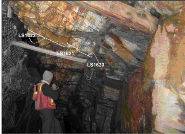
Figure 8. Sampling historic underground workings at the 100 Level of the Little Squaw Mine. The back (roof) of the adit is massive white quartz vein, with a banded quartz-gold footwall zone (right) of the Little Squaw Vein. The vein is 4 feet thick at this location and the view is along strike looking west. The white bars represent sample areas. Samples LS1621 and LS1622 contained only trace amounts of gold, and sample LS1620 assayed 89.12 ounces of gold per ton. Photo provided by James Barker and Little Squaw Gold Mining Co.
