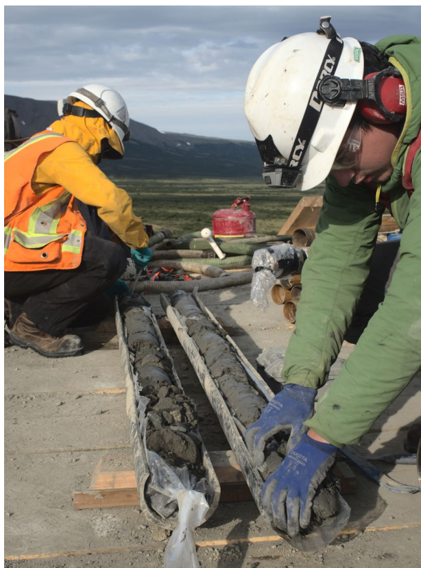
Photo 3. Preparing sonic drill core for logging at the Graphite One project. Photo: Graphite One Inc.
