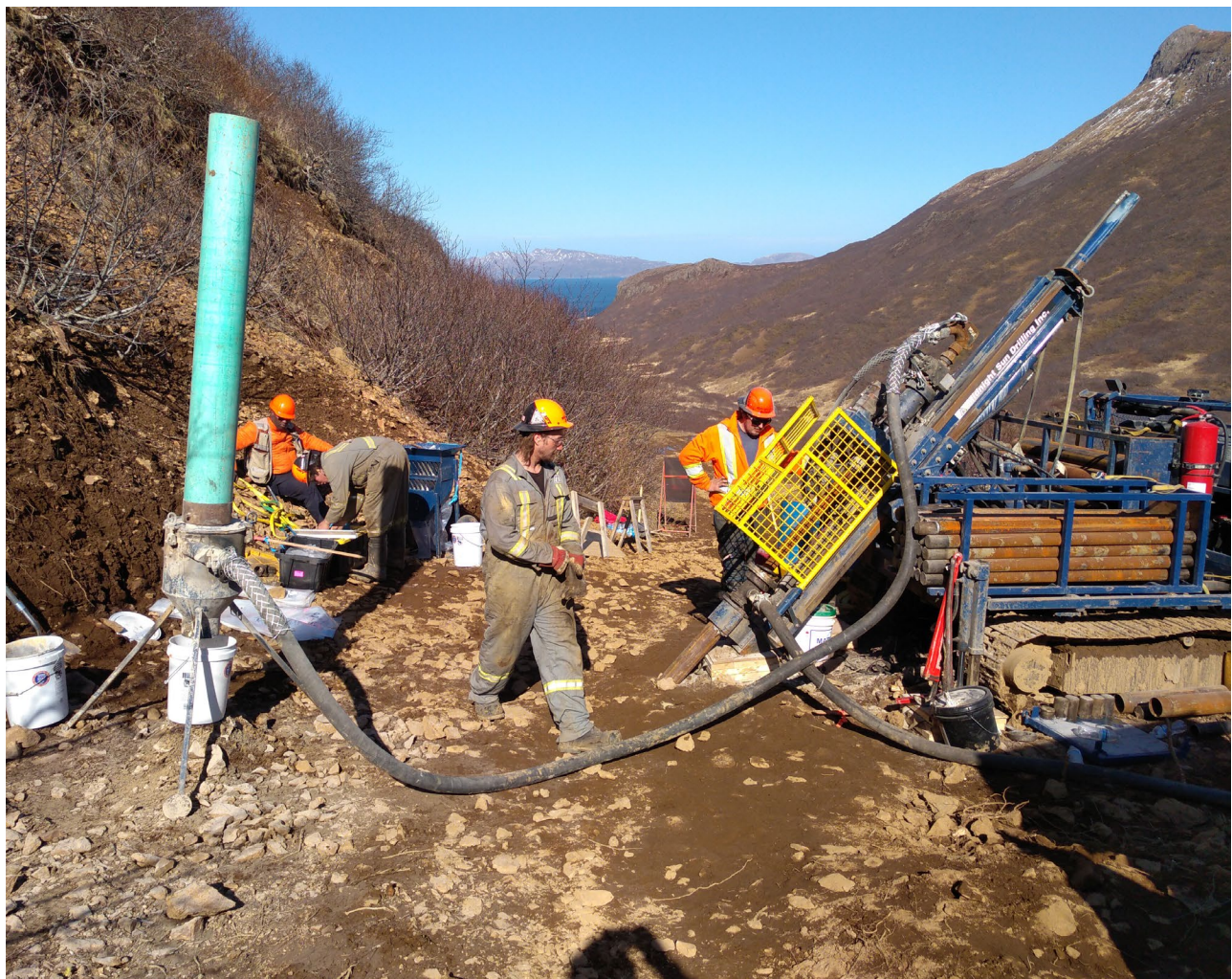
Photo 1. Midnight Sun RC rig at the SH-1 vein on the Unga project. Photo provided by HelioStar Metals Ltd.
