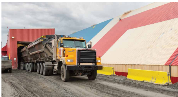
Photo 2. Truck passing through air wash system after unloading concentrate from the Red Dog Mine at the concentrate storage building at the Red Dog port site. Photo provide by Teck Alaska Inc.
