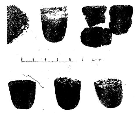
Figure 3-Coke products from selected Alaskan coals (top) and coal blends (bottom)
