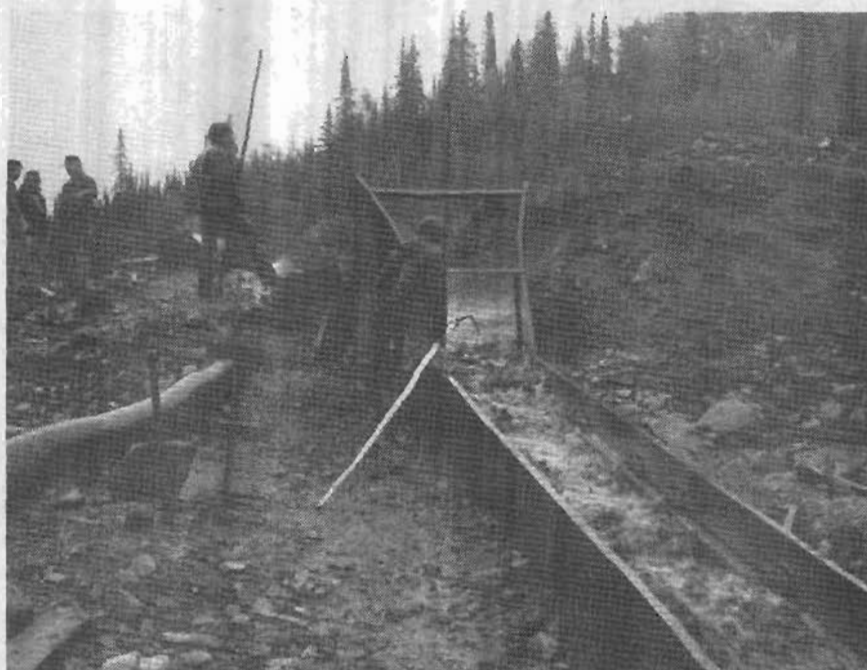
Side loading sluice box arrangement, with rock raker in foreground.
