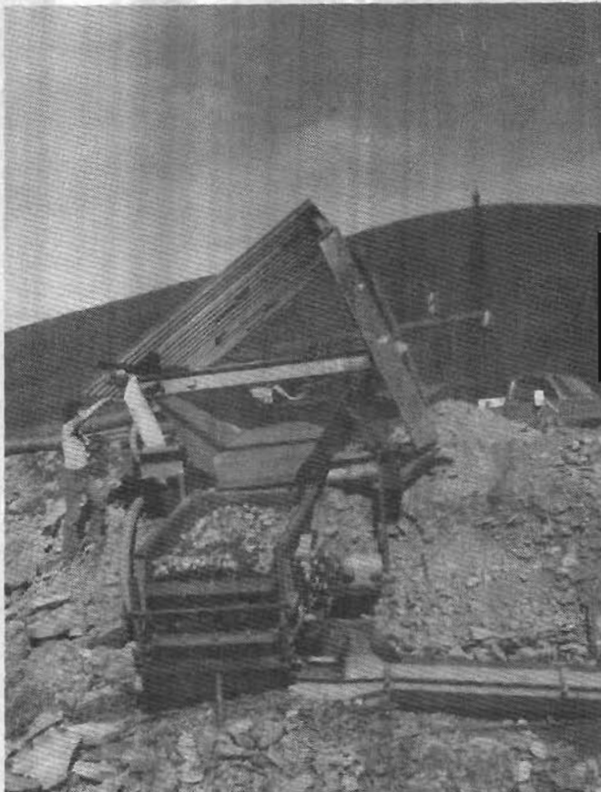
Sloping grizzly and shaking screen.
