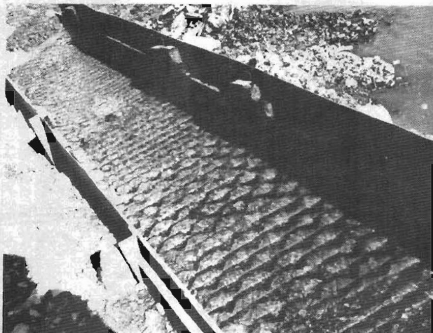
Fig. 11 - Notched angle-iron riffles used by Robert Wilkinson on Miller Creek
