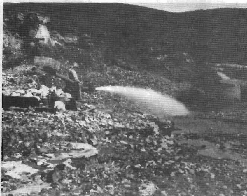
Fig. 1 - Hydraulicking into sluice box, F.E. Co. Operation at Engineer Creek
