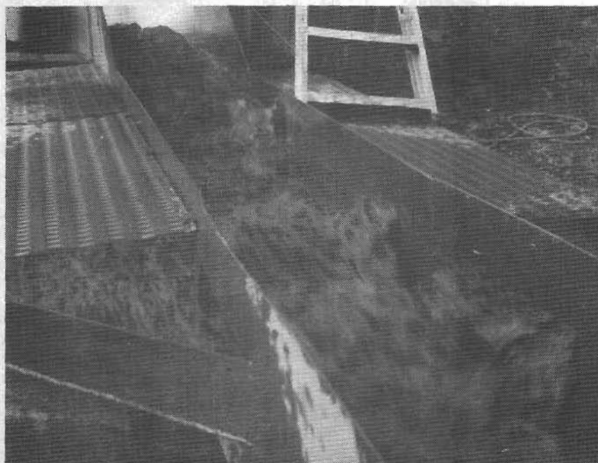
Turbulence in main and side sluices of a Ross box.
