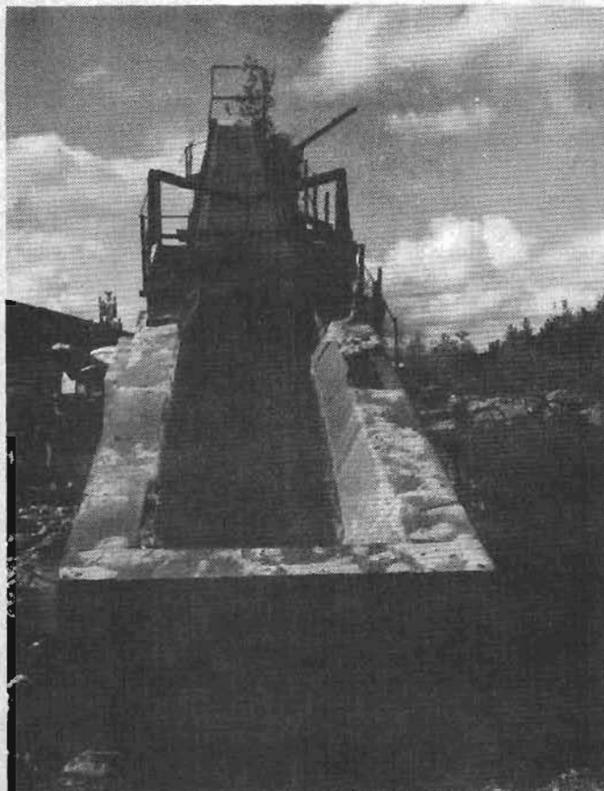
Hopper and conveyor system for elevated sluice box type of operation.
