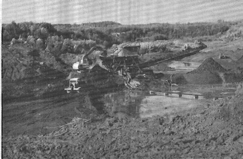
Figure 4. Loading the washing plant with a hydraulic excavator.
