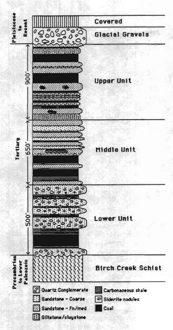
Figure 4. Generalized stratigraphic section, Jarvis Creek coalfield, Alaska
