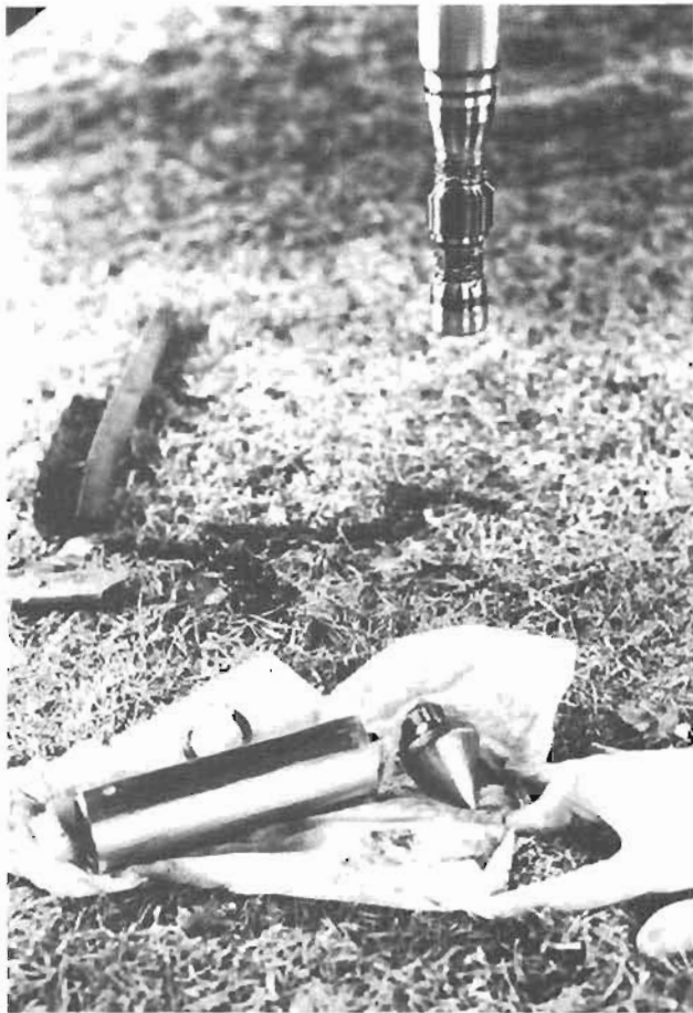
Figure 16. Closeup of cone assembly with cone and friction sleeve removed to show instrumentation.
