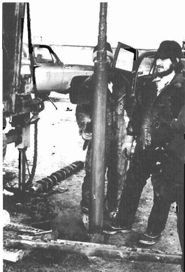
Figure 4. Recovery of 12.7-cm (5-in.) diameter, 1.52-m (5-ft-) long Shelby-tube sampler from borehole site B-5 (for location see fig. 3).
