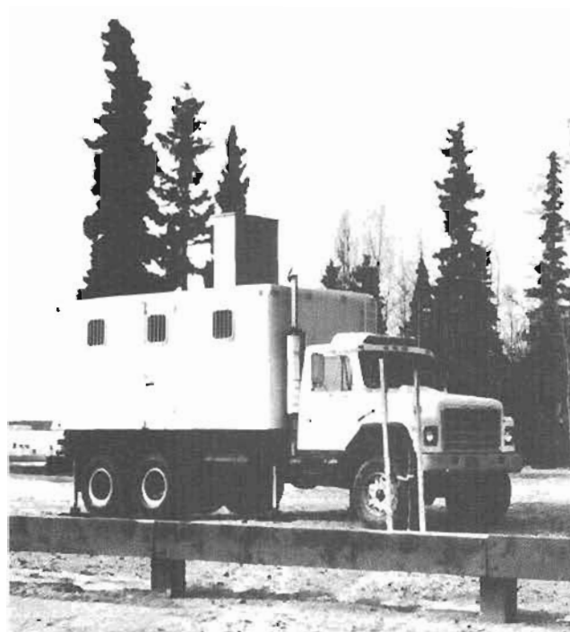
Figure 14. Truck-mounted cone-penetrometer test (CPT) system at the LA-C-3 sounding site.
