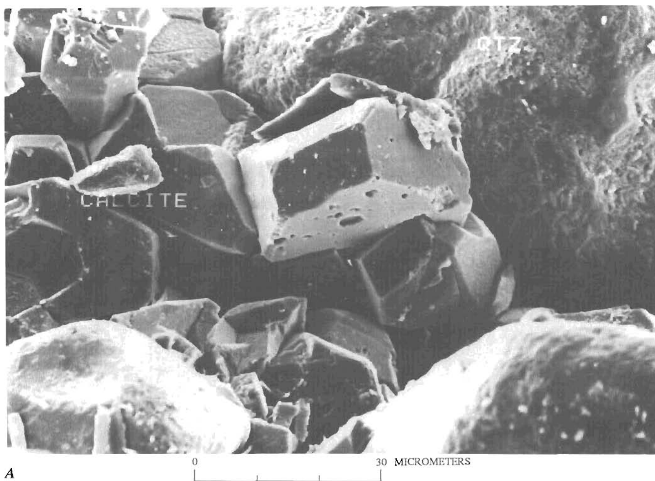
Figure 7. Scanning electron microscope photomicrographs of calcrete from Great Kobuk Sand Dunes. A , Well-developed secondary calcite grains. B , Typical glaciofluvial features. Qtz, quartz.
