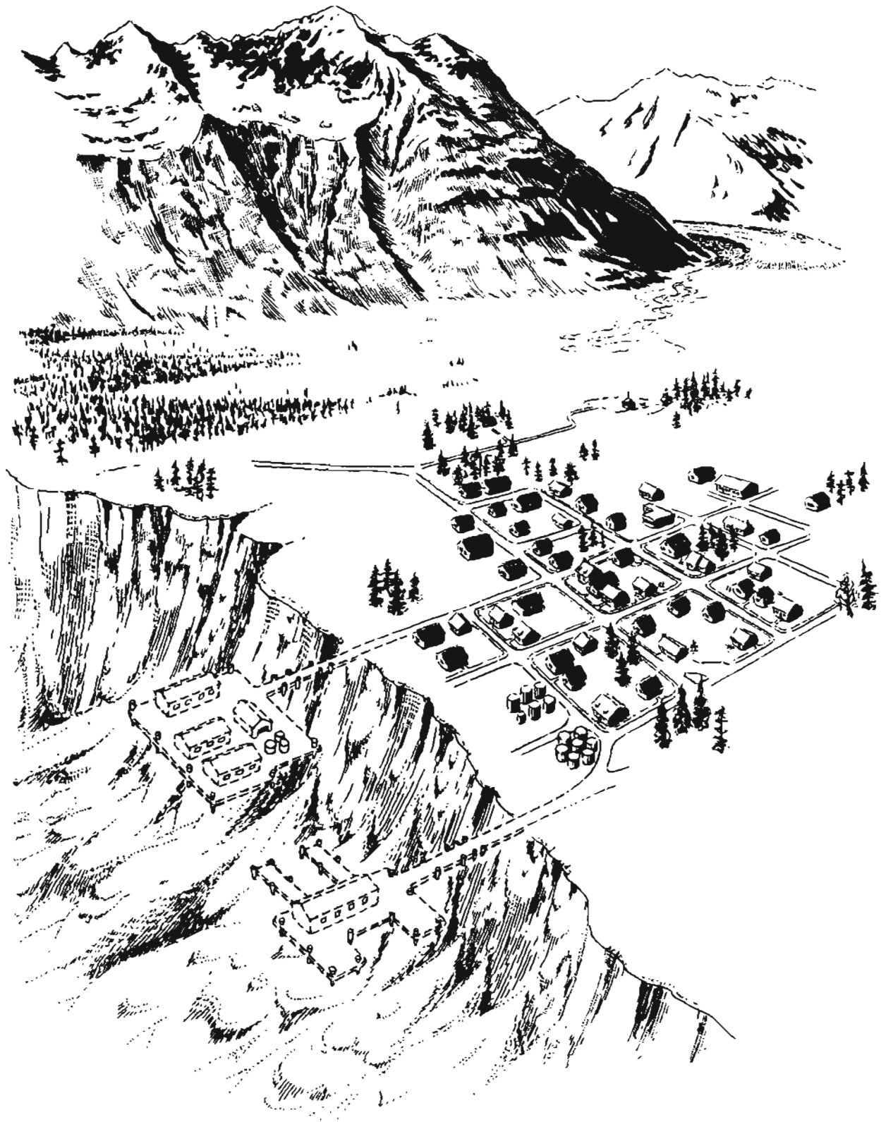
Figure 13. Submarine landslide area at Valdez (from Coulter and Miliaccio, 1966). The dashed lines indicate the dock area destroyed by the landslide.
