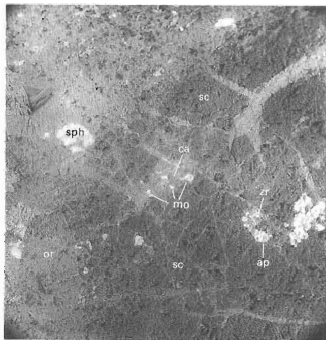
Figure 6. Scanning electron microscope backscattered-electron image of HM rock sample CDP-92-29. A grain of scapolite (sc) is veined by calcite (ca) and potassium feldspar (or). Molybdenite (mo) occurs within a calcite vein in the upper left corner of the scapolite grain. Accessory minerals include sphene (sph), apatite (ap), and zircon (zt). Field of view is approximately 2 mm.
