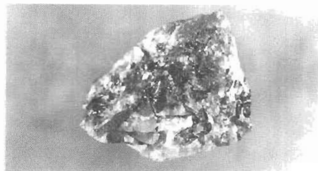
Figure 3. Fragment of HM rock sample CDP-92-29. Molybdenite occurs throughout the fragment. At bottom center, molybdenite occurs on planes in calcite. Sample is approximately 3 cm across. Photograph by Lewis V. Thompson
