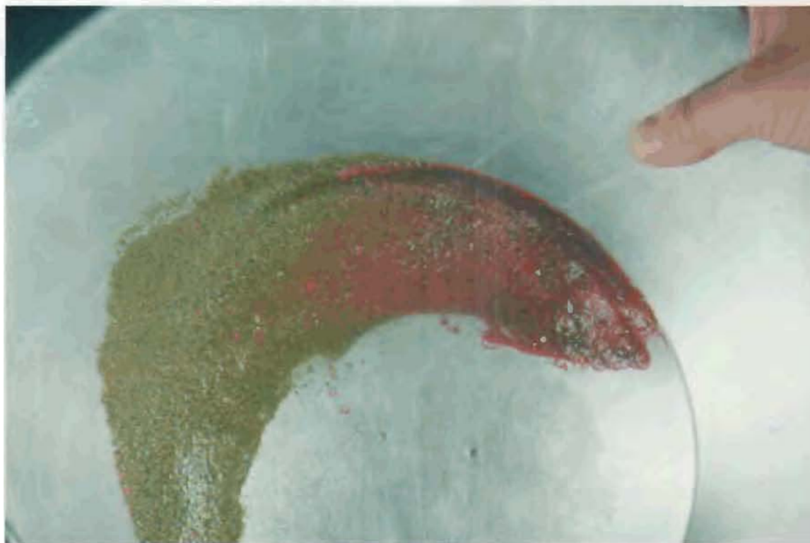
Figure 13. Heavy-mineral sample in a gold pan showing abundant cinnabar particles.
