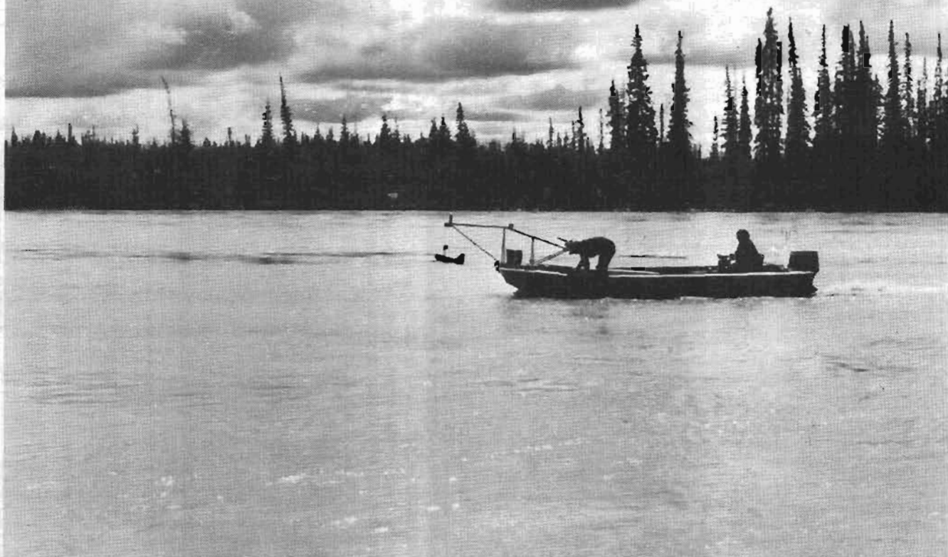
Suspended-sediment sampling in the Tanana River near Fairbanks.
