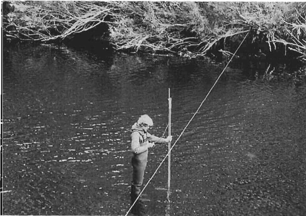
Figure 10. FWS scientist uses Prick current meter to measure discharge of Little Black River in Yukon Flats NWR. Water flow is measured at intervals along tag line to produce a profile of total discharge at this point in river. Photograph from FWS files.
