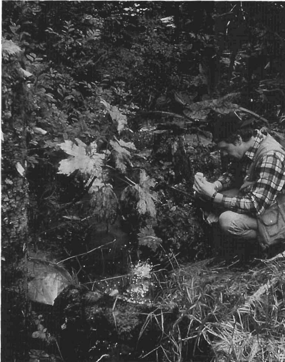
Figure 2. USBM geologist measures pH level of discolored water below main waste-rock dump at the Juneau-area Peterson Mine, which produced small amounts of gold from quartz-arsenopyrite ore between 1905 and the early 1920's. Although iron-stained, the water was only slightly acidic at pH 6.5. The USBM was evaluating the mine as part of the FS program on abandoned mine hazards in the Tongass National Forest. Photograph from USBM files.
