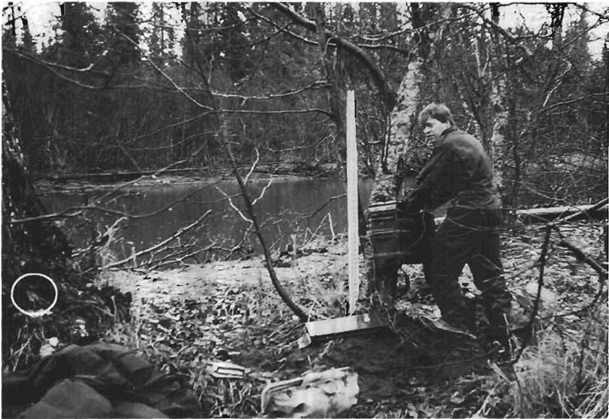
Figure 4. FWS scientist downloads data from electronic meter at Fox River stream gauging station in Kenai NWR. Flagging in base of tree at left (circled) indicates high-water mark from September 1995 flood. Photograph from FWS files.
