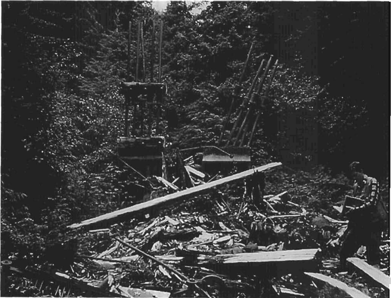
Figure 22. USBM geologist sketches ruins of 10-stamp mill at Lucky Chance Mine at headwaters of Salmon Creek, 21 kilometers south of Sitka. The USBM was evaluating the mine as part of the FS program on abandoned mine hazards in the Tongass National Forest. Photograph from USBM files.
