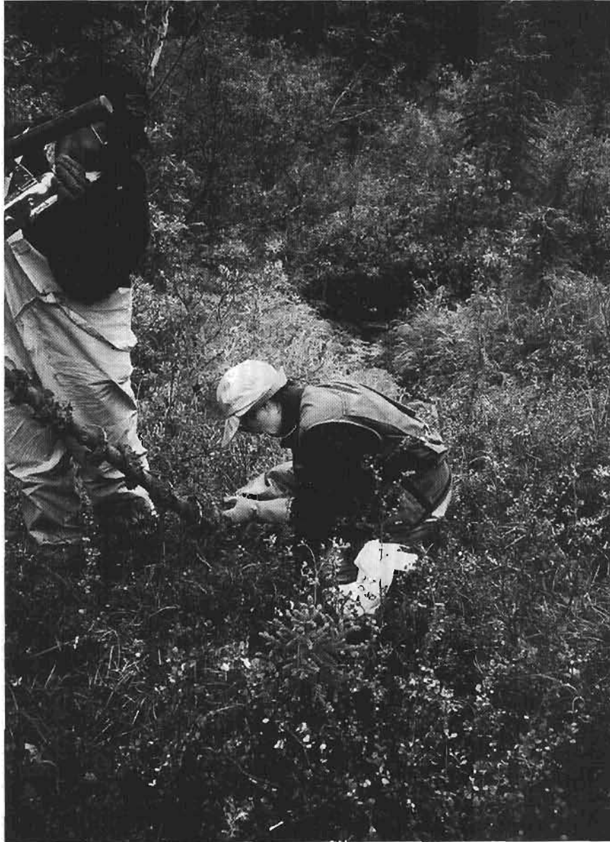
Figure 17. Using gas-powered auger, Calista Native corporation personnel sample soils in Stuyahok River-Flat Creek area of southwestern Alaska. The USGS and Calista are working together to assess the mineral resources of the area. Photograph by E.A. Bailey, USGS.
