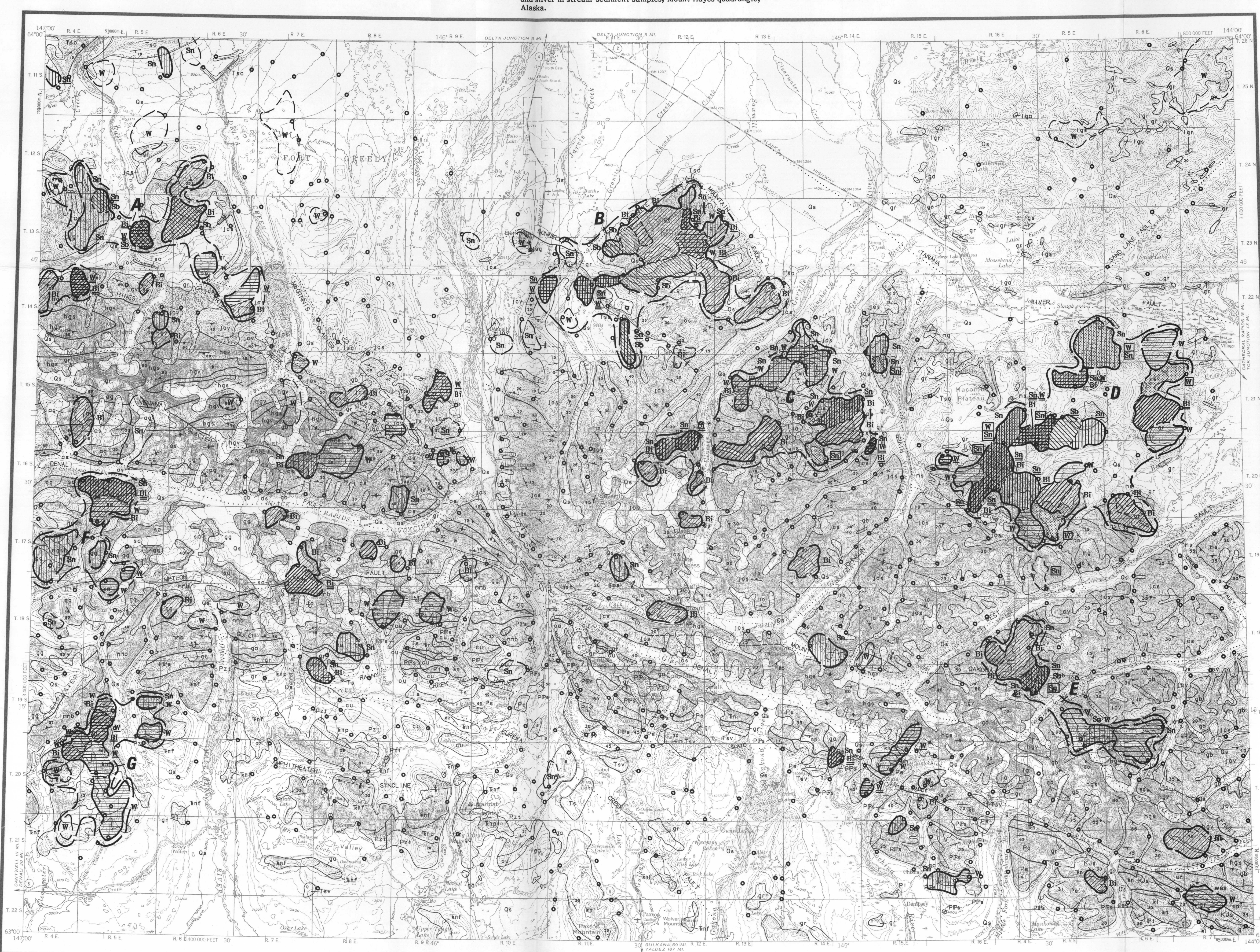
Map D.—Th, tungsten, antimony, and bismuth in heavy-mineral concentrates and tin and tungsten in stream-sediment samples, Mount Hayes quadrangle, Alaska.
