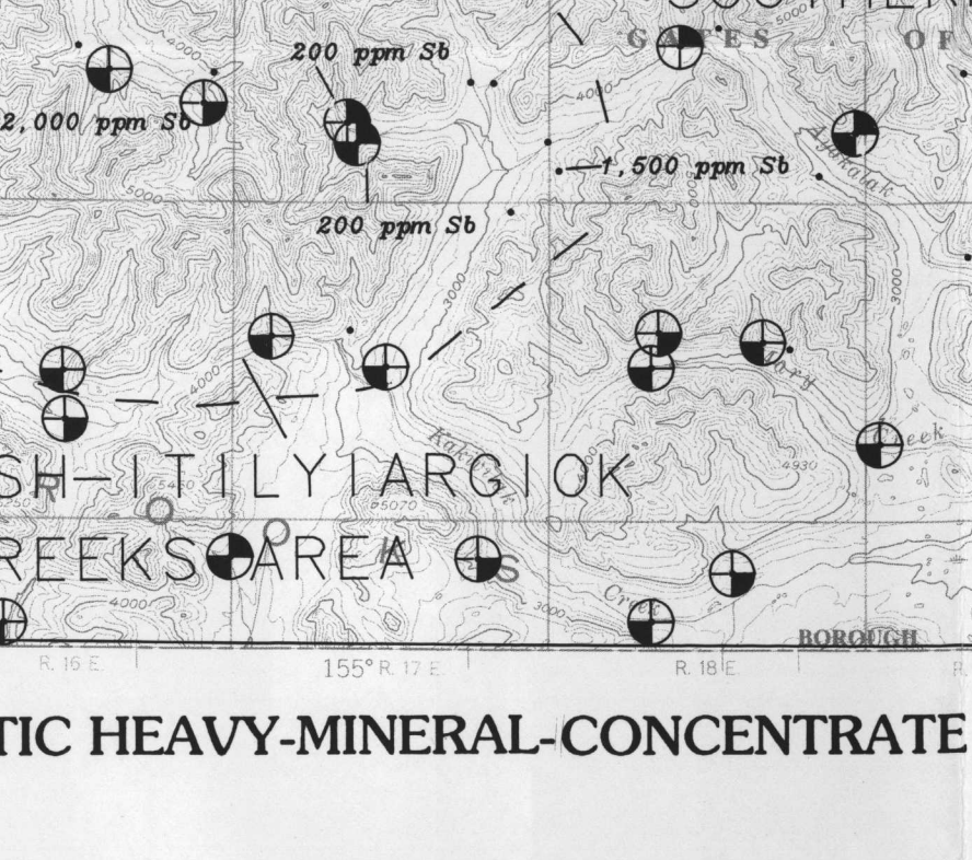
MAP B. DISTRIBUTION OF NONMAGNETIC HEAVY-MINERAL-CONCENTRATE SAMPLES CONTAINING ANOMALOUS CONCENTRATIONS OF Ag, Cu, Pb, Sn, AND Zn
