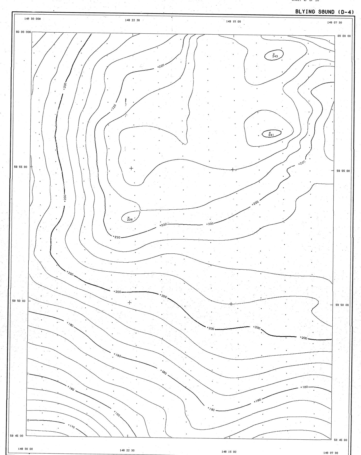
CONTOUR INTERVAL ..... 5.0 GAMMAS DATUM ..... 55,417.81 GAMMAS INSTRUMENT. . . . GEOMETRICS G-803 PROTON MAGNETOMETER
