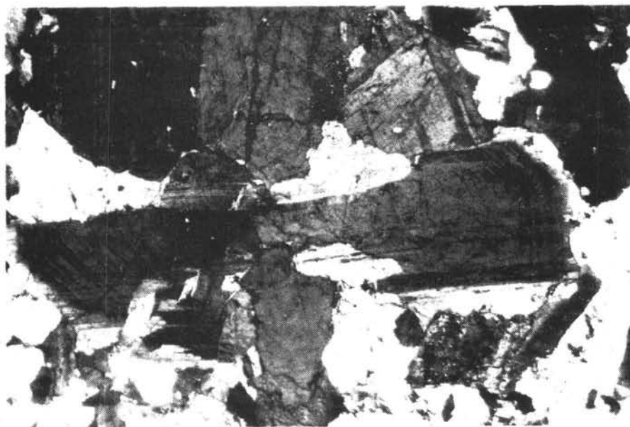
Figure 26. Photomicrograph of above specimen; note oscillatory zoning in large plagioclase phenocrysts (12X).
