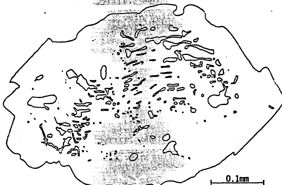
Figure 4. Outline of a single pyrite grain (polished section 205). Small blebs within the pyrite grain are chalcopryrite, tennantite, and bornite. The pyrite grain is surrounded by chalcopryrite.
