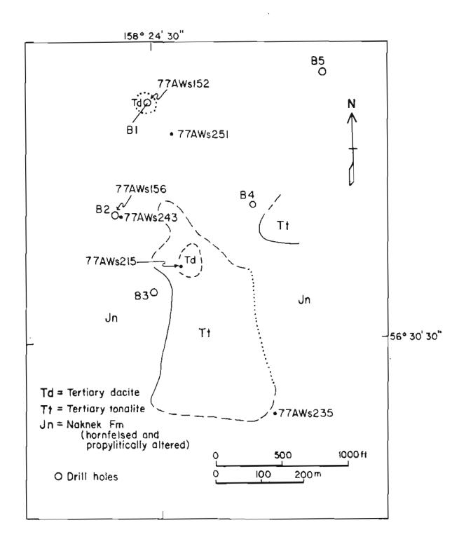
Figure 4. Sketch geologic map of the Bee Creek prospect, showing location of drillholes and dated samples.
