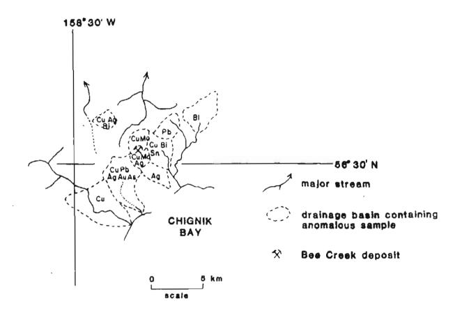
Figure 3. Associations and zoning of anomalous metals in nonmagnetic heavy mineral concentrates from stream sediments near the Bee Creek deposit. Anomalous values in ppm for each element are as follows: Ag >2, As >500, Au >20, Bi >20, Cu >700, Mo >10, Pb >150, Sn >20, Zn >500. W, >500, was not anomalous in this system.
