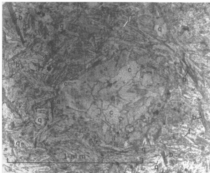
FIGURE 19.—Photomicrograph of biotite basalt, from locality 5½ miles northwest of Sleetmute, north of Kuskokwim River. Relict pyroxene phenocryst in center of picture is completely altered to carbonate (c) and antigorite (a); groundmass includes plagioclase feldspar (f), biotite (b), and quartz (q). Plain light.
