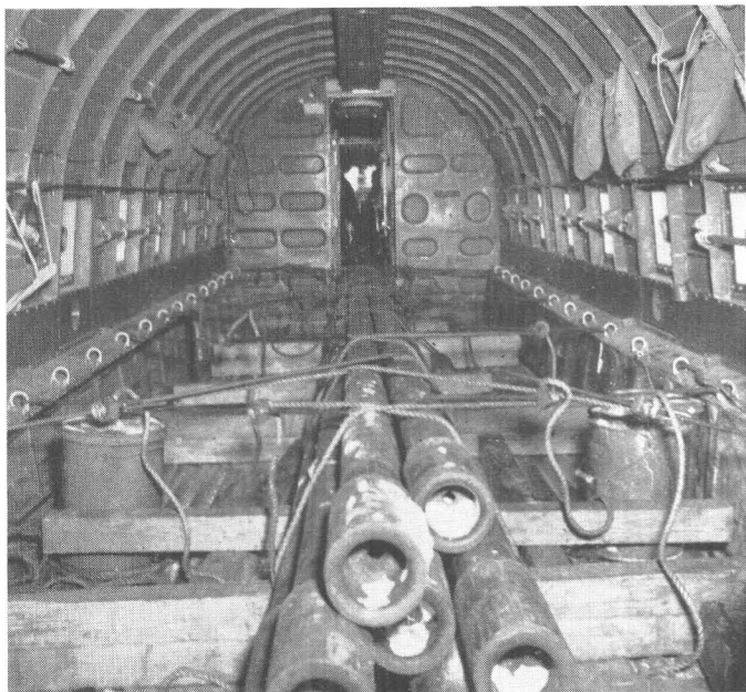
FIGURE 16.—Manner of carrying drill pipe in aircraft for freighting between Barrow and Umiat in April 1945. Photograph by U. S. Navy.
