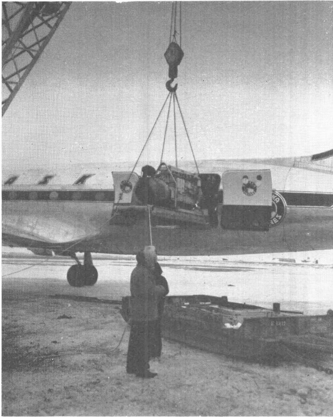
FIGURE 49.—Loading 75-kw generator aboard a C54 aircraft at the Barrow airfield. Photograph by U. S. Navy.
