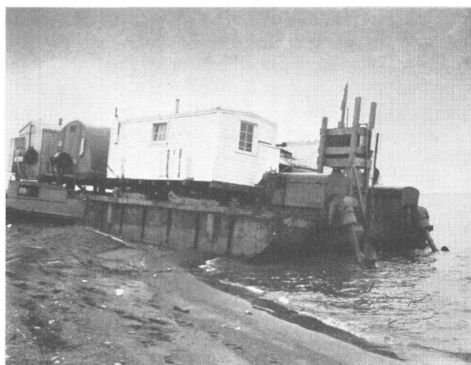
FIGURE 44.—Camp set up on barge for waterborne seismic operations. Photograph by U. S. Navy, September 1948.
