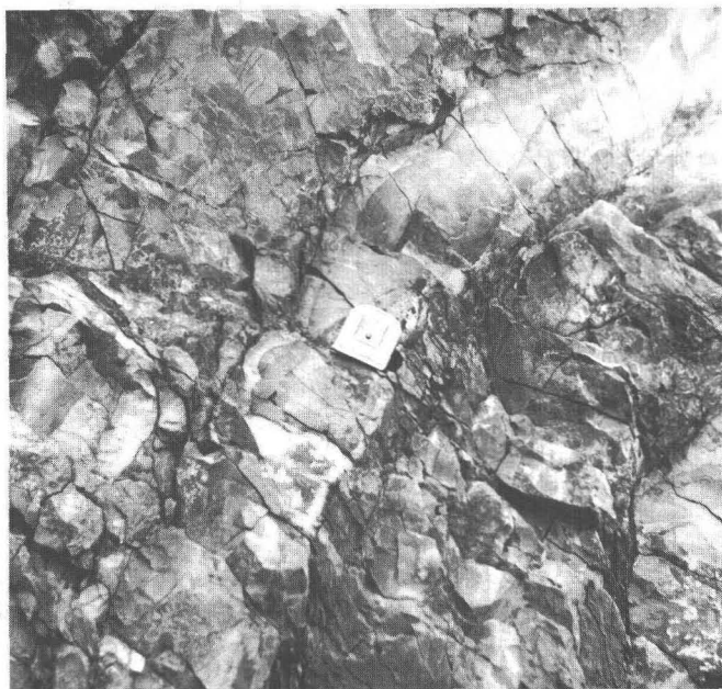
FIGURE 21.—Bedding characteristics and outcrop aspect of some of the mudstone of the Kisimilok Formation. Thin- to medium-bedded clayey mudstone in which bedding is expressed chiefly as color banding (of various hues of gray). Note also the lack of distinctively resistant strata and the conchoidal fracture. Straight edge of tape case is 2 inches long.
