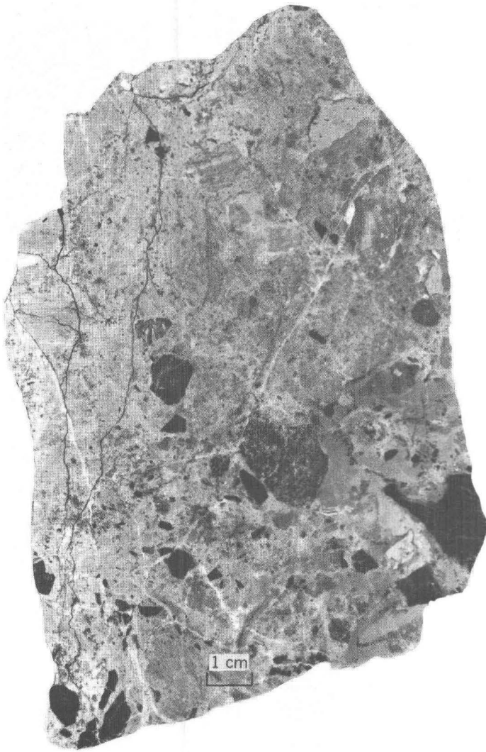
FIGURE 9.—Texture and clast size in dolomitized sedimentary breccia in the Kogruk(?) Formation. The clasts are dark-colored chert and lighter colored dolomite, in a matrix of medium crystalline dolomite and only minor relict(?) calcite micrite.
