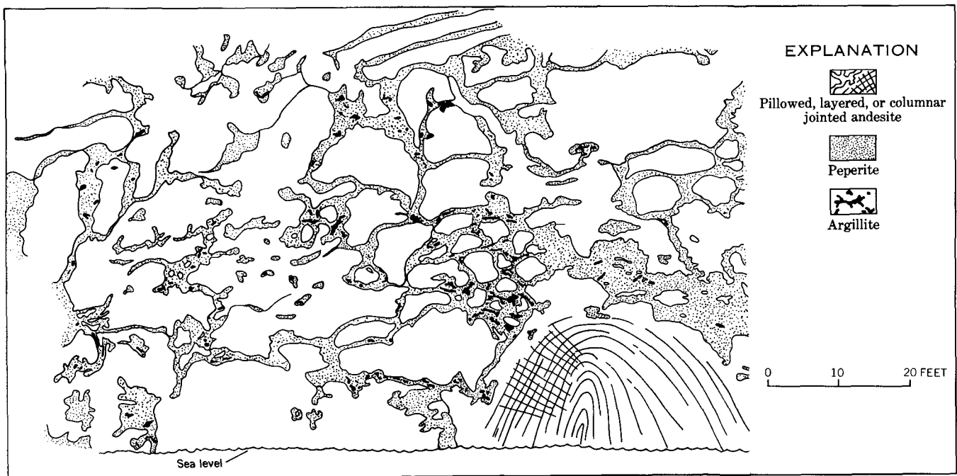
FIGURE 19.—Pillowed lava in sea cliff exposure 1½ miles west of tip of Lance Point, Unalaska Island; drawn from several photographs. Baked deformed argillite occurs in center of peperite masses. Lava necks typically connect pillows with each other and with a layered lava pod at the lower right.
