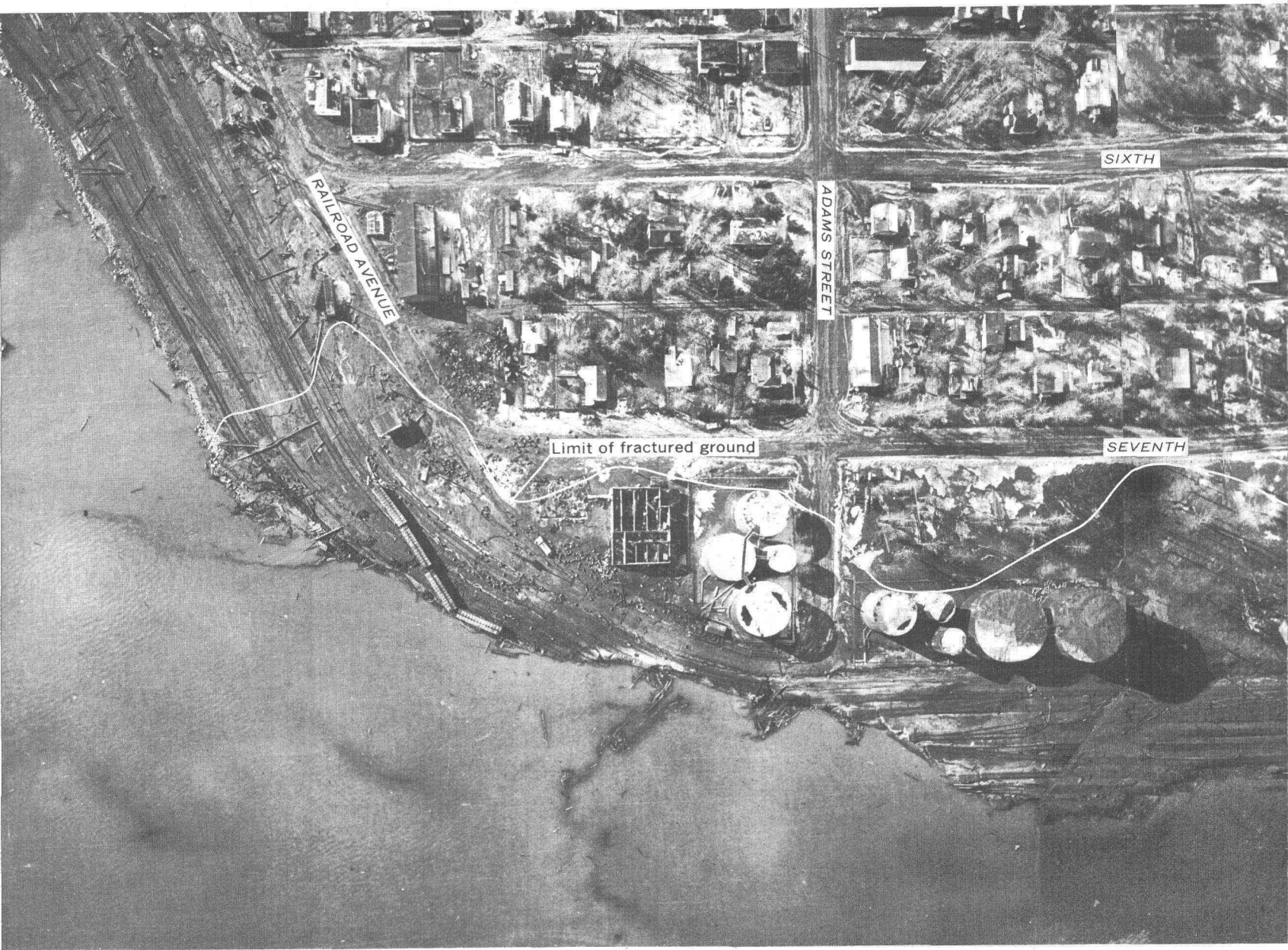
3. Aerial view of the southern part of the Seward waterfront showing extent of ground fracture and earthquake damage. Photographed by U.S. Navy.
