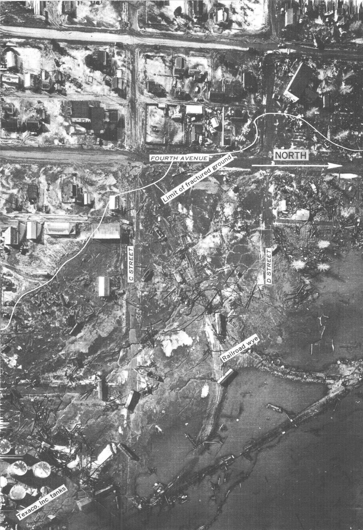
4. Aerial view of the northern part of the Seward waterfront showing extent of fractured ground and earthquake damage. Photograph by U.S. Army; mosaicked by U.S. Geological Survey. Index map (upper left) shows relation of figures 3 and 4.
